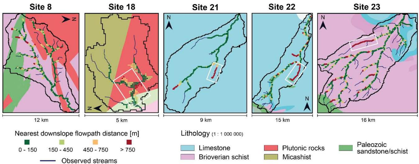
**Figure 8.** For the 5 sites corresponding to  $r_{optim} > 2$ , representation of the observed stream network on top of the simplified geological map (1:1 000 000 scale), with the downslope flowpath distances of the simulated seepage areas projected to the observed streams. For site 8, differences are larger on the plutonic rocks. For the other sites, the white square identifies the area where differences are the largest.
