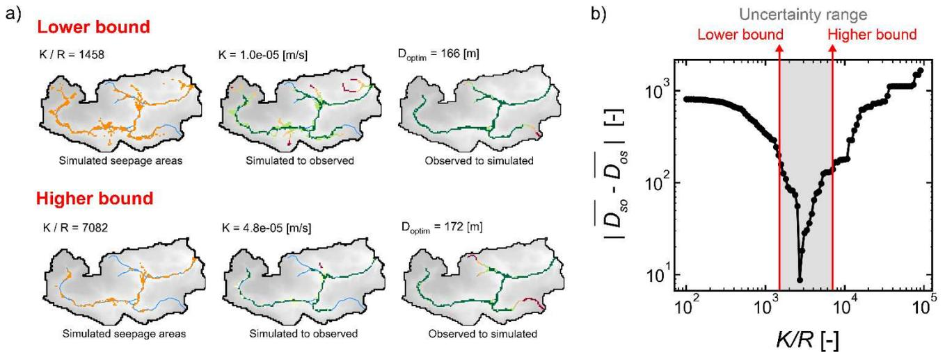
**Fig. B1.** For the Canut catchment (site 6), a) 2D map views of simulated seepage areas and nearest downslope flowpath distances (simulated to observed and observed to simulated) for the two  $K/R$  at the bounds of the uncertainty (lower and higher), and b) the objective function based on the developed performance criteria obtained.
