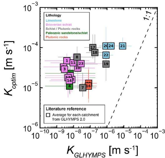
Fig. C1. Comparison of  $K_{optim}$  obtained for the 24 catchments with values of the literature provided by the GLHYMPS 2.0 global permeability map (Huscroft et al., 2018),  $K_{GLHYMPS}$ , averaged over each catchment.
