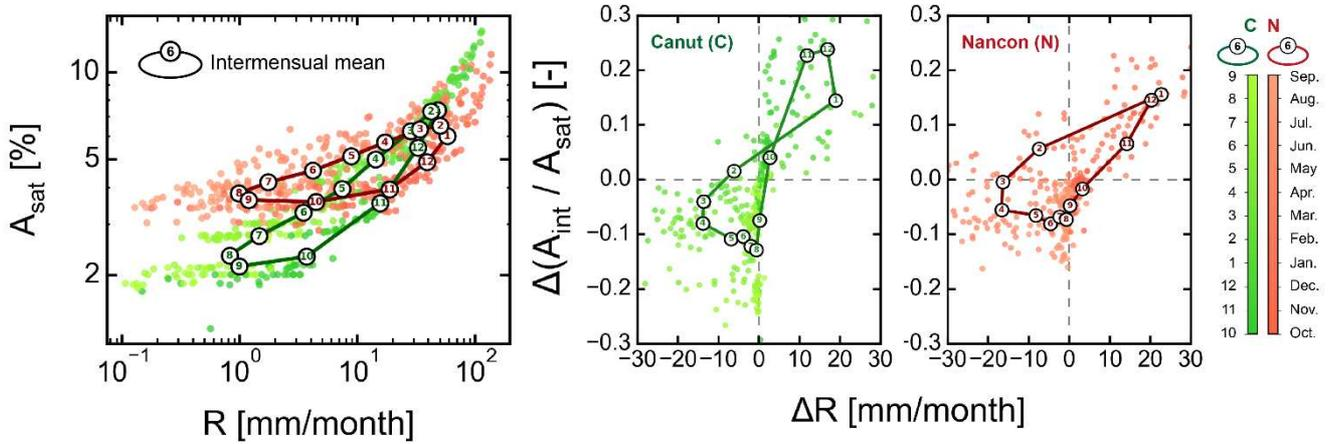
325 **Figure 5.** a) Simulation results of the proportion of the total water saturated area  $A_{sat}$  at the catchments scale as a function of the recharge applied to the model. b) Variation in the proportion of intermittent water saturated area  $A_{int}$  as a function of recharge variation  $\Delta R$ . Each colored point corresponds to a value of a month of the year over the period 1960-2019 with the black line corresponding to the intermonthly average.
