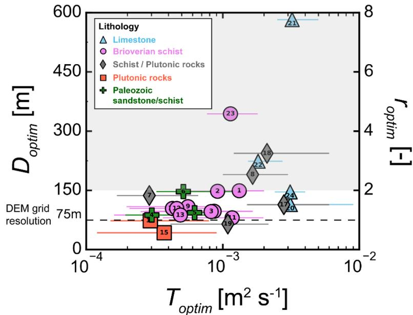
Figure 6.  $D_{optim}$  and  $r_{optim}$  criteria as functions of  $T_{optim}$  estimated for the 24 sites. The optimal transmissivity  $T_{optim}$  is obtained by considering  $K_{optim}$  and the mean saturated aquifer thickness  $d_{sat}$  computed. The shaded area corresponds to sites with  $r_{optim} > 2$ . The DEM resolution is 75 m and the aquifer thickness is 30 m. The error bars correspond to the estimated  $T_{optim}$  considering the DEM resolution as an uncertainty indicator.
