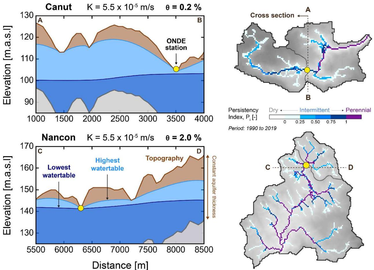
Figure 4. a) Cross section of the maximal (high water) and minimal (low water) groundwater level simulated. b) Persistence index map for the Canut and Nancon watersheds calculated from simulation results ranging from 1960 to 2019.
