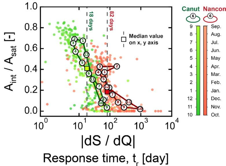
335 **Figure 6.** Proportion of intermittent water saturated area  $A_{int}$  in relation to the total  $A_{sat}$  at the catchment scale as a
