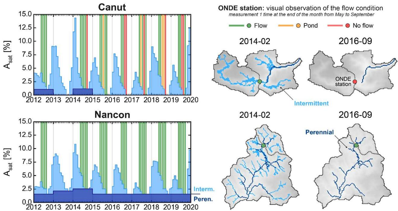
280 **Figure 3.** a) Location of the two studied catchments, the Canut and the Nancon. b) Proportion of water saturated area simulated at sub-catchment scale : upstream of the ONDE station (discontinuous and continuous hydrographic network). In the background, the type of flow observed at the ONDE station (once a month from May to October since 2012, with one missing year in 2013). c) Mapping of the simulated stream network for February 2014 and in September 2016.
