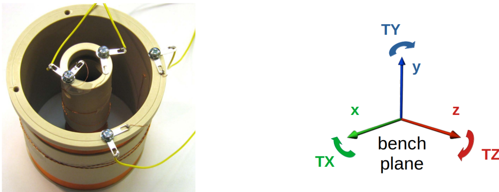
Figure 4.14.: On the left, a picture of a pair of LVDT coils is shown [83]. The primary coil is the one in the center and the secondary one is the cylinder containing it. On the right, the reference system of the benches coordinates is shown.
