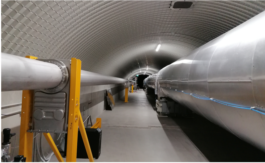
Figure 4.9.: Picture of the filter cavity tube, parallel to the North Virgo arm.
