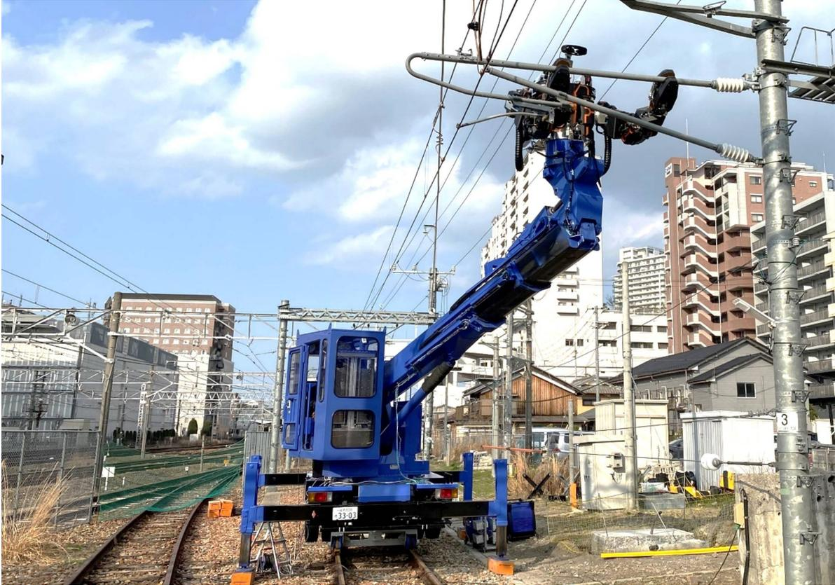
FIGURE 1.7 – Rei shiki Robot operating metallic parts over a railway, credit: The Japan Time
