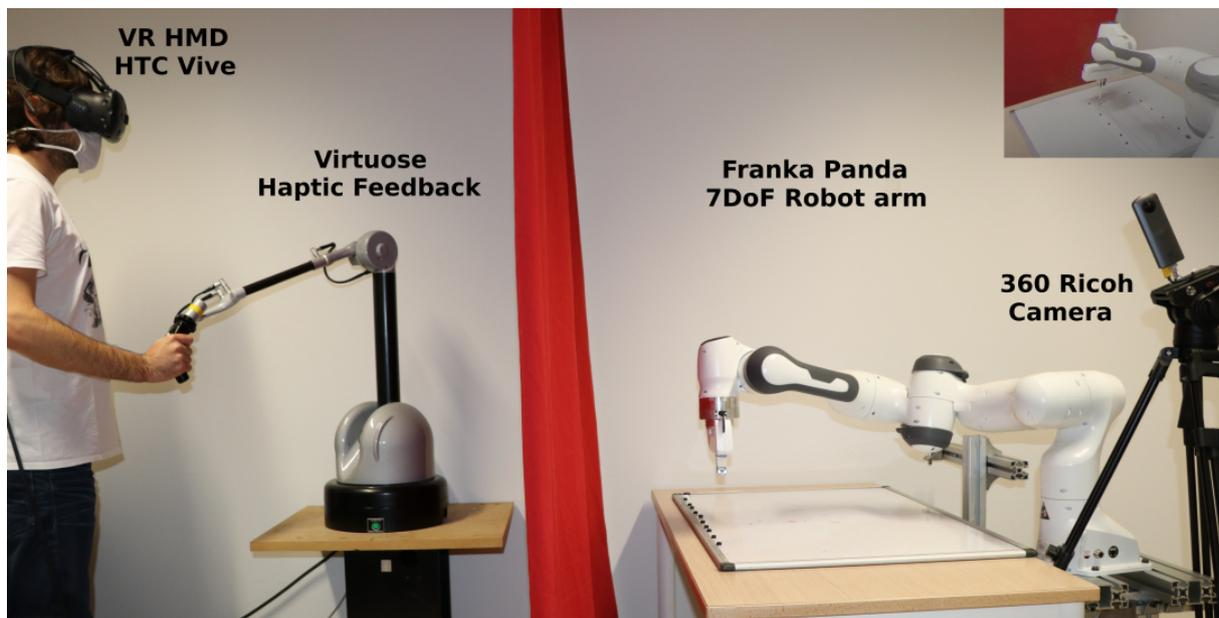
FIGURE 3.1 – Embodied teleoperation setup. Our setup consists of a Virtuose haptic device and a Franka Panda robot. The operator wears a head mounted display and operates the robot using the haptic device. He is provided with a first person visual display from a camera placed above the Franka. The controller utilized to help him guide the trajectory and impedance of the robot is explained in Sect. 3.4.
