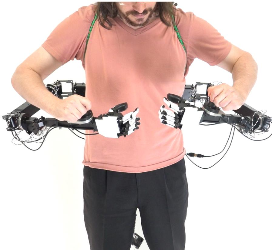
**FIGURE 2.1** – The Co-Limbs user interface uses force sensors and admittance control to enable a user to intuitively move through force sensors levers and use the otherwise non-backdrivable wearable robotic arms.
