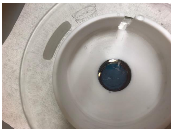
Figure 3.3. Picture of the spontaneous film of gold nanoparticles at the surface of ethylene glycol
