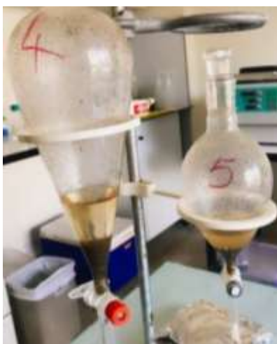
Figure 14 Separating microplastics by density separation in a separatory funnel
