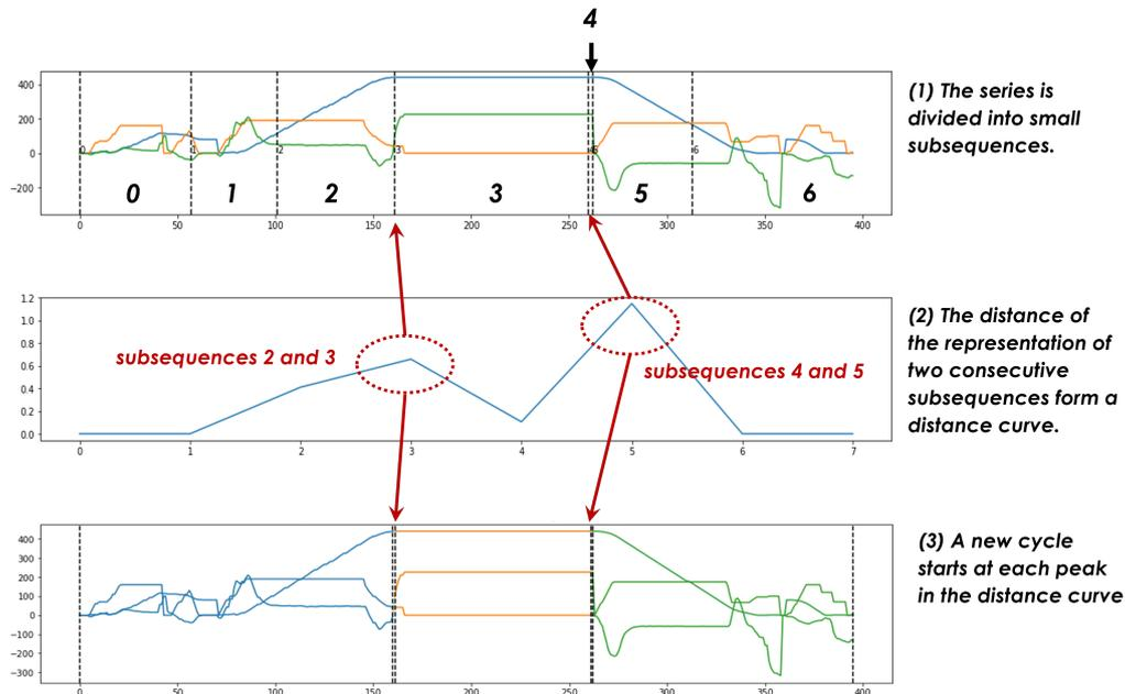
FIGURE 4.14: Three steps of the Autoencoder-based extractor
