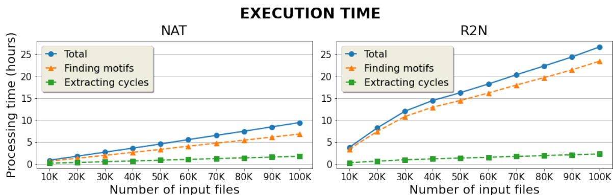
FIGURE 4.25: Execution time of InterCE on NAT and R2N data sets, from 10^4 to 10^5 files
