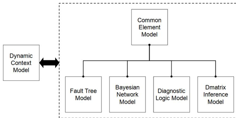
FIGURE 2.14: Structure of diagnostic models in IEEE AI-ESTATE [101]
