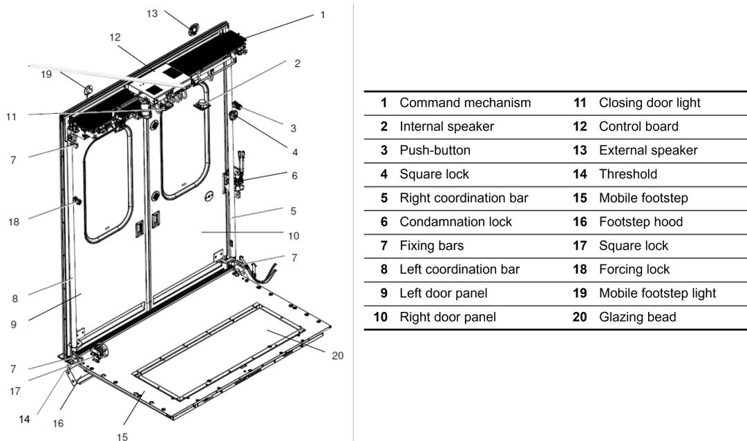
FIGURE 3.2: Components of a PAS with a mobile footstep
