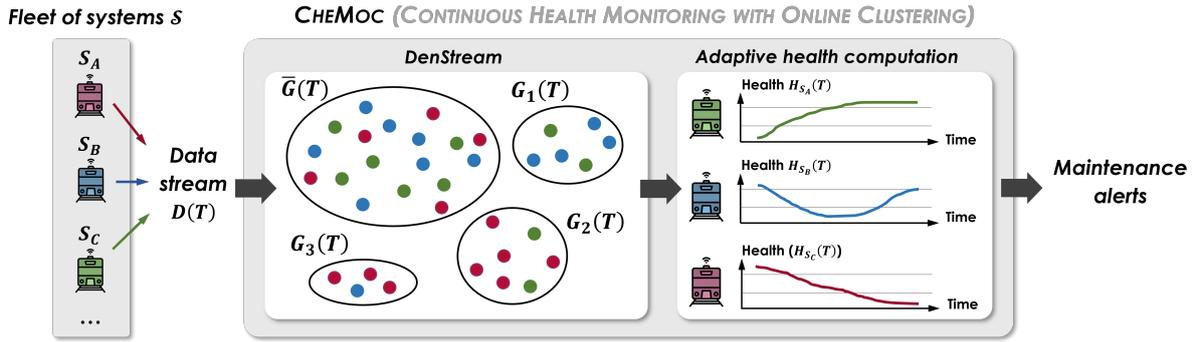
FIGURE 6.1: From a stream  $D(T)$  containing the data from all the systems in the fleet, CheMoc uses a modified version of DenStream to update the clusters on new data, then computes the health score  $H_{S_m}(T)$  of each system  $S_m$  adaptively.
