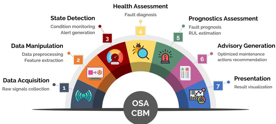
FIGURE 2.11: The standard architecture proposed by OSA-CBM.
