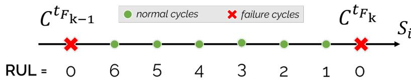
FIGURE 7.2: From a cycle at a known moment of failure ( $C_{t_{F_k}}$ ), we increment the RUL backward, starting from the value 0 at  $C_{t_{F_k}}$ , until we reach the cycle of the previous known moment of failure ( $C_{t_{F_{k-1}}}$ ). The annotation stops one cycle before  $C_{t_{F_{k-1}}}$ .
