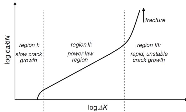
FIGURE 2.8: The crack growth divided in three regions [222].
