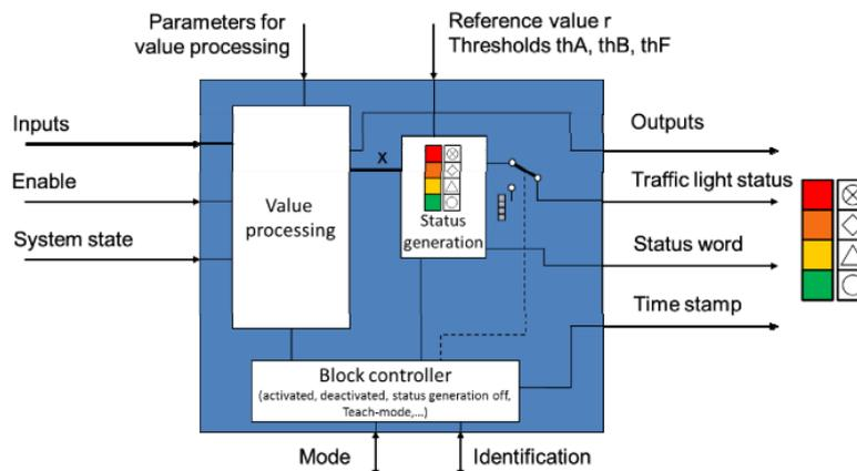
FIGURE 2.12: A functional block of VDMA 24582 [231].
