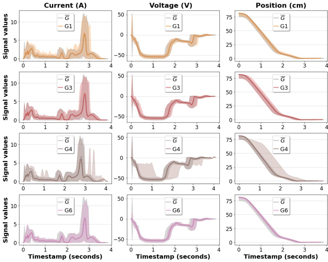
FIGURE 6.10: Visualization of the profiles of  $G_1$ ,  $G_3$ ,  $G_4$ , and  $G_6$  via the current, voltage, and position measurements. Thick lines are the profiles, and colored regions are the envelopes of the variables.
