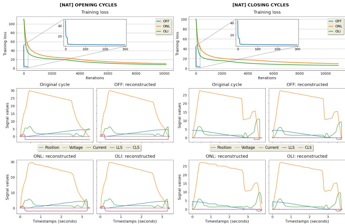
FIGURE 5.6: Training losses and reconstruction of one example cycle of OFF, ONL, and OLI models on NAT cycles
