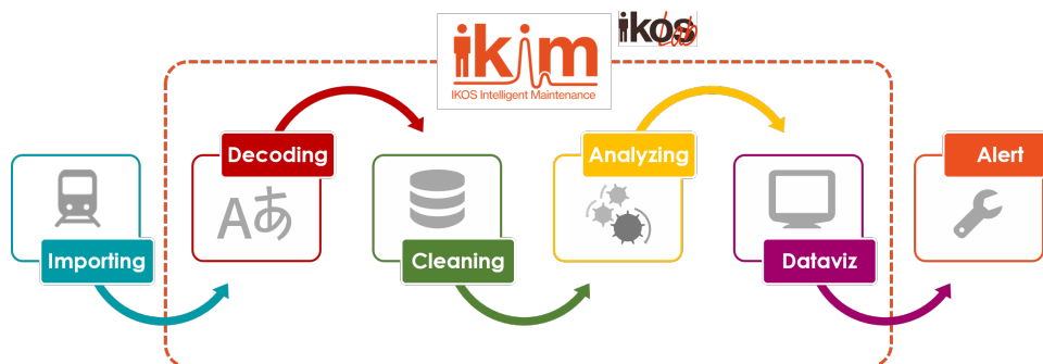
FIGURE 8.5: The IKIM platform dedicated to big data processing for railway predictive maintenance, under development at IKOS Consulting
