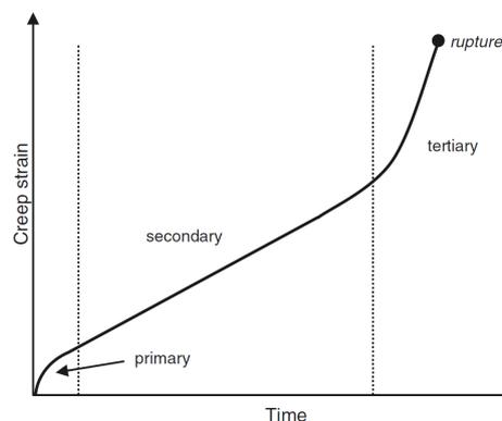
FIGURE 2.7: Three regions of the creep curve [222].
