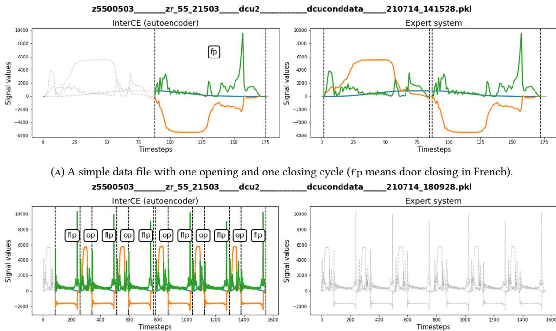
(A) A simple data file with one opening and one closing cycle (fp means door closing in French).
