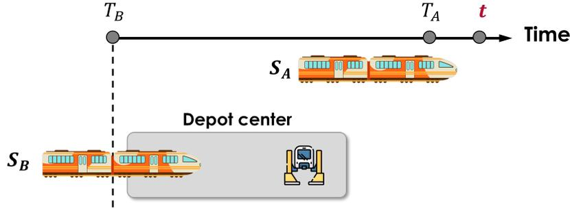
FIGURE 6.3: The system  $S_B$  enters a depot center at  $T_B$  and stops producing data, while the system  $S_A$  continues operating until  $T_A$ . The most recent data of  $S_B$  are not indexed at  $t$  but at  $T_B$ .
