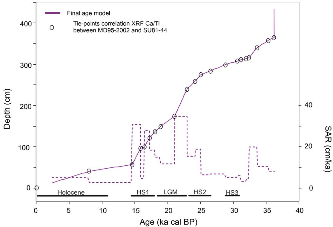
Figure IV-S 1. Age model of core SU81-44 based on synchronization of XRF-Ca/Ti ratios (full purple line) with cores MD95-2002 and BOBGEO-CS05 (Zaragosi *et al.*, 2006; Toucanne *et al.*, 2021; Depuydt *et al.*, 2022). Sediment accumulation rate (SAR; dashed purple line) in SU81-44.
