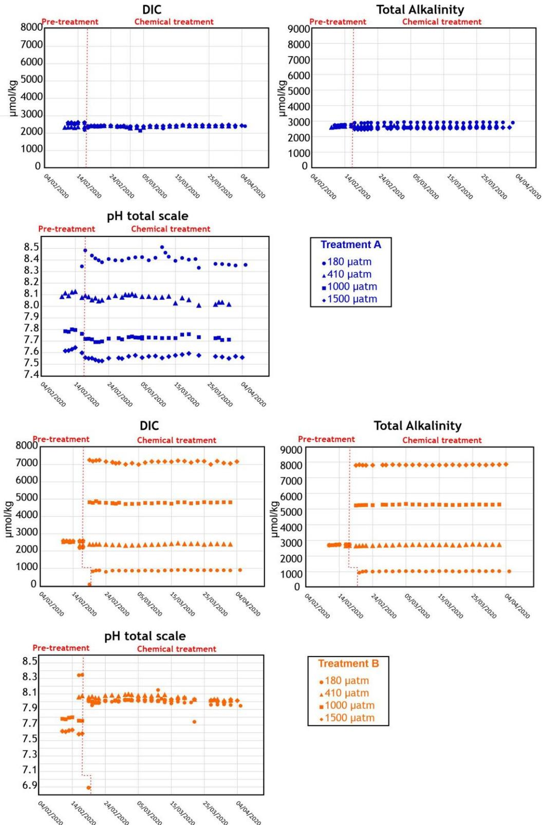
Figure VI-S 3. Graphics showing the three measured parameters of the C-system during the experiment.
