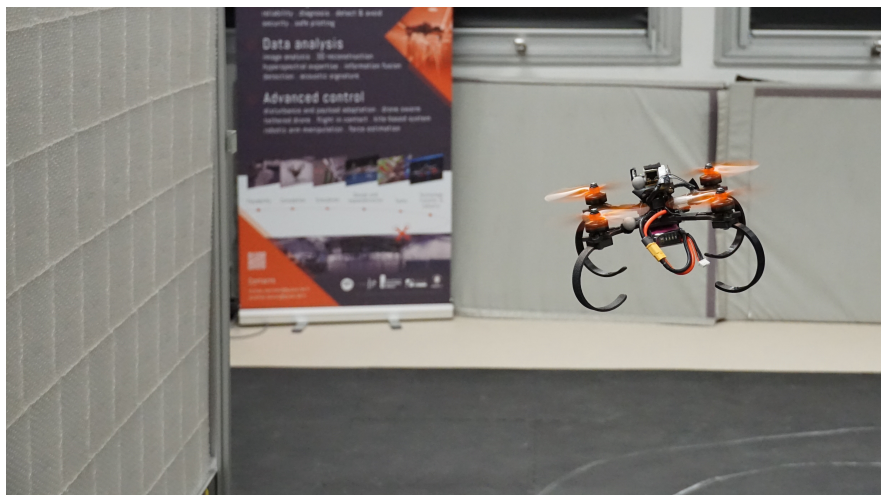
Figure IV.7: The Kopis quadrotor facing the wind indoor tunnel.
