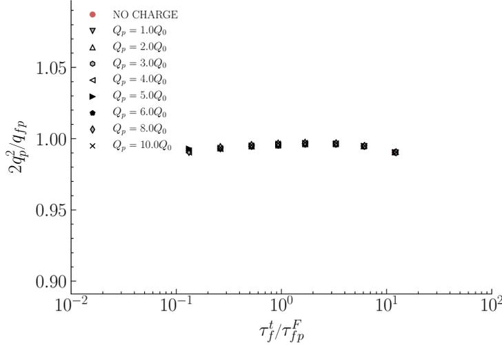
**Figure 5.8:** Effect of electrostatic interactions on the ratio between the particle kinetic energy and the fluid-particle velocity covariance with regard to particle inertia for various levels of electric charge.
