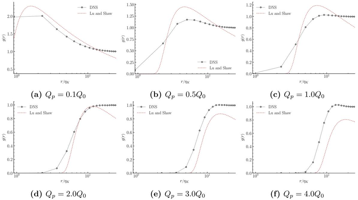
**Figure 5.44:** *RDFs of the lighter particles compared with Lu & Shaw (2015) model of Eq. (5.17) for various levels of electric charges. We observe an agreement on the trend of the evolution of RDFs for weak electric charges, one of the hypotheses of the cited model.*
