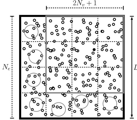
**Figure 4.9:** Computational domain  $\Omega$  of length  $L$  is discretized in  $N_e$  cells per direction. For each particle  $p$  (black dot), its neighborhood  $V_p$  (bold gray) spans  $2N_v + 1$  cells to each direction. Pseudo-particles (gray circles) are defined for every cell  $\Omega_k$  outside of  $V_p$ .
