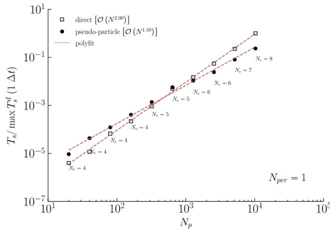
**Figure 4.12:** The simulation time ( $1 \Delta t$ ) for direct and pseudo-particle algorithm ( $N_v = 1$  and  $N_{per} = 1$ ) normalized by its maximum value (for direct algorithm) is plotted against an increasing number of particles for optimal number of cells  $N_e^{opt}$ .
