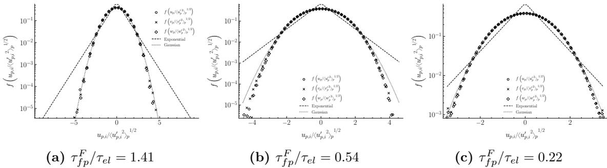
**Figure 5.48:** *PDF of the three components of particle velocities for various levels of particle inertia and  $Q_p = 5Q_0$ . The distributions are perfectly Gaussian (see Eq. (3.55)).*
