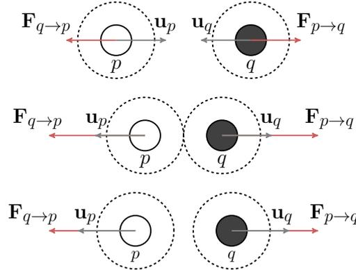
**Figure 4.16:** *Schematic of a Coulomb collision of two like-charged particles and notion of Coulomb diameter. Particle diameter  $d_p$  is depicted with a solid dark gray circle, while (fictitious) effective Coulomb diameter with a dashed black circle.*
