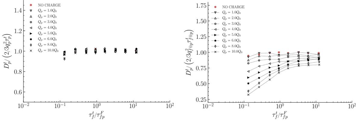
**Figure 5.28:** Particle dispersion coefficient models' validity for various levels of electric charges and particle Stokes numbers. To the left,  $2/3 \times q_p^2 \tau_p^t$  seems to give a good estimate and to the right  $2/3 \times q_{f@p}^2 \tau_{f@p}^t$  seems to overestimate of  $D_p^t$  for like-charged particles.
