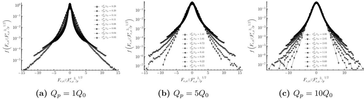
**Figure 5.32:** Effect of particle inertia on the PDF of the  $x$ -axis component of electrostatic forces for  $Q_p = [1, 5, 10] Q_0$ . Increasing particle inertia narrows the range of electrostatic forces, while increasing electric charge widens it.
