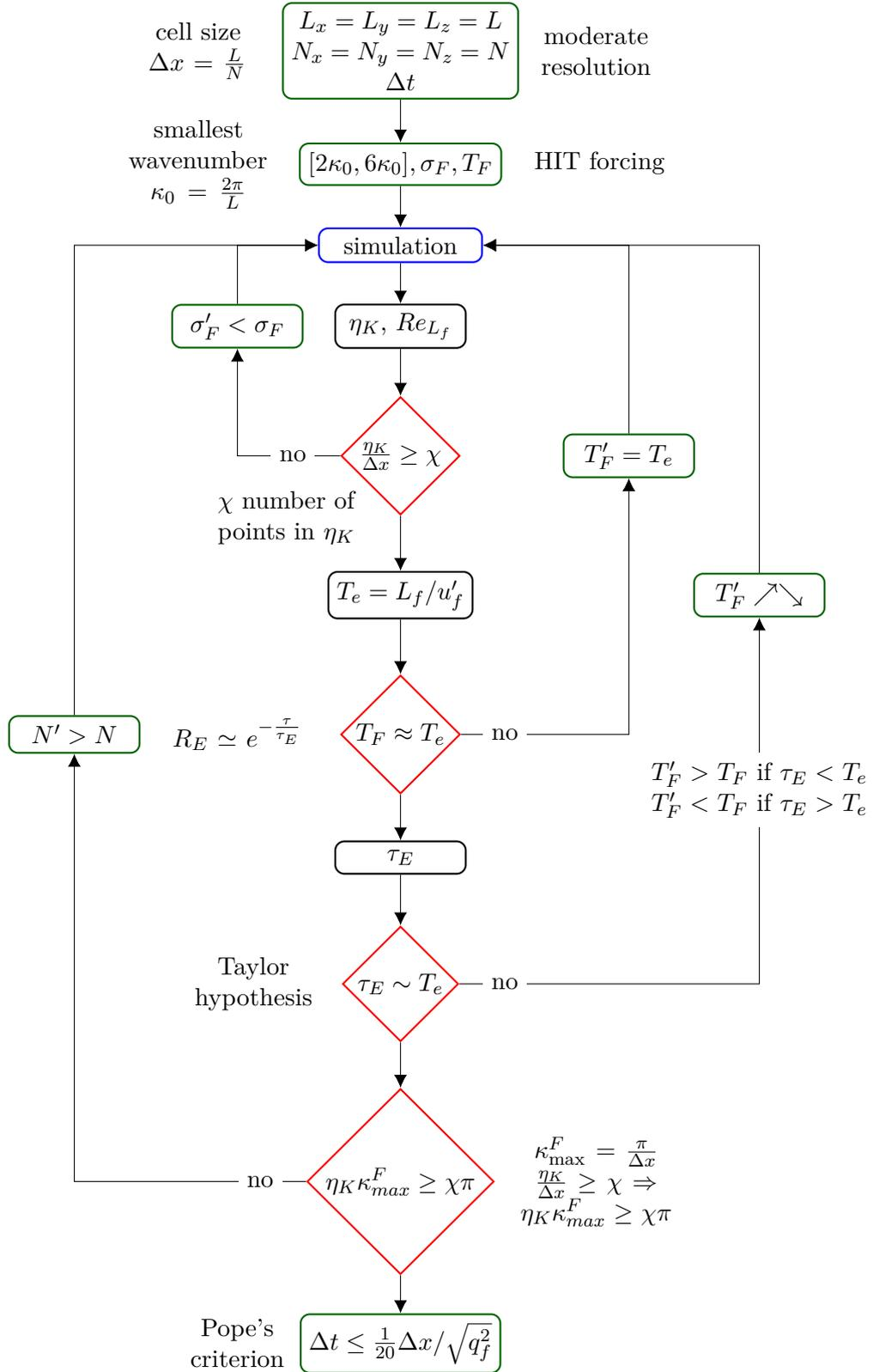
**Figure 2.1:** Flowchart for the calibration of resolved stationary HIT. Green color denotes a choice/modification for the value of the corresponding variable, red denotes checking the satisfaction of a criterion, black denotes the calculation of a statistic variable and blue the simulation of turbulence.
