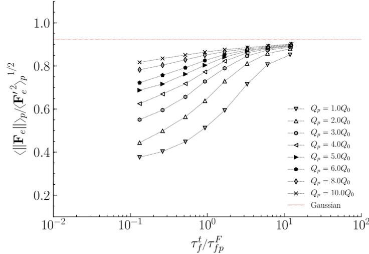
**Figure 5.31:** Effect of electrostatic interactions on the shape of the PDFs of electrostatic forces via ratio  $\langle \|\mathbf{F}_e\| \rangle_p / \langle \mathbf{F}_e'^2 \rangle_p^{1/2}$ . The horizontal line corresponds to its theoretical value for Gaussian distribution (Fede, 2004, Wang *et al.*, 1998).
