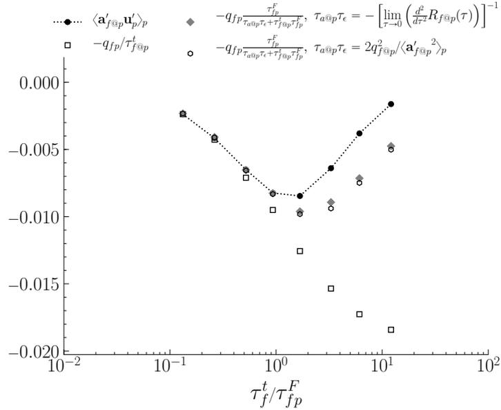
**Figure 5.9:** Comparison between DNS results (●) and the predictions of the Langevin model (□) and the introduced stochastic model (◆, ○) of the fluid acceleration - particle velocity covariance  $\langle \mathbf{a}'_{f@p} \mathbf{u}'_p \rangle_p$  with regard to particle Stokes number for  $Q_p = 5Q_0$ .
