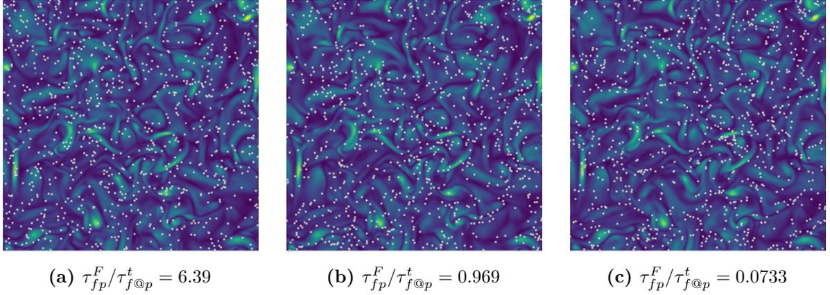
**Figure 3.14:** Instantaneous snapshots of the turbulent vorticity field and the particle distribution for various levels of inertia for  $\Delta x = L_f$ .
