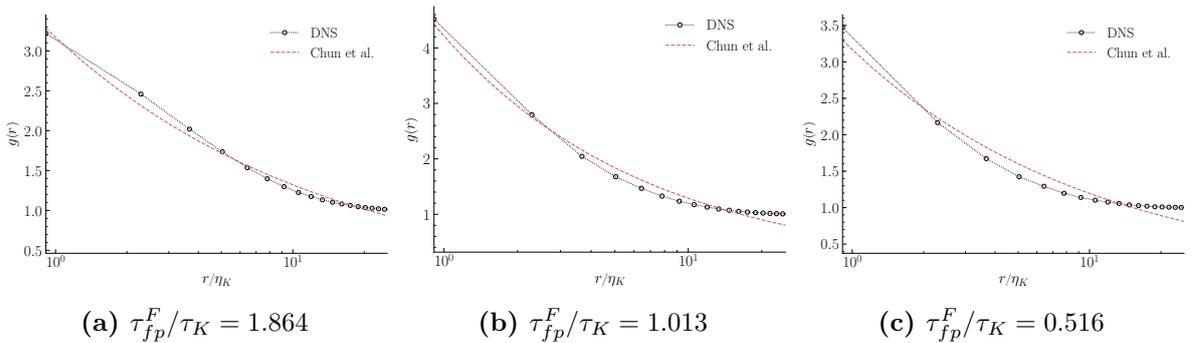
**Figure 3.23:** RDFs of inertial particles having low Stokes numbers,  $\tau_{fp}^F/\tau_K$ . The red dashed line corresponds to Eq. (3.52) that has been fitted via non-linear least squares optimization.
