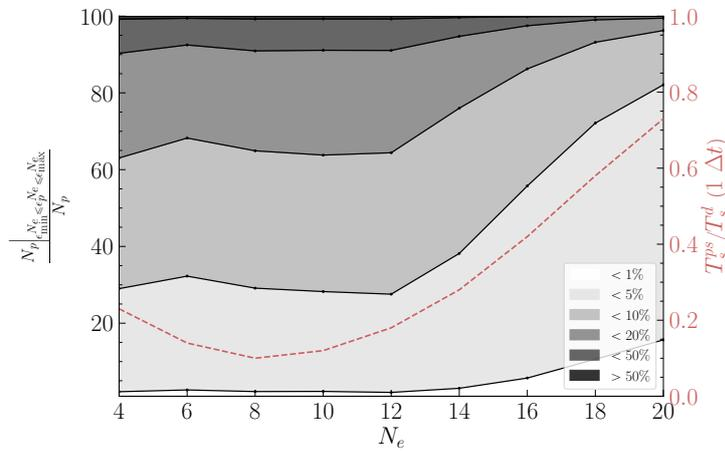
**Figure 4.13:** Relative approximation error distribution with regard to number of cells  $N_e$  of pseudo-particle algorithm for one time-step and  $N_p = 10,000$ . A different shade of gray is attributed to the percentage of particles for which the approximation error is between 0%, 1%, 5%, 10%, 20% and 50%. The red dashed line shows the simulation time of the pseudo-particle algorithm ( $N_v = 1$ ,  $N_{per} = 1$ ) normalized by that of the direct algorithm for the same case.
