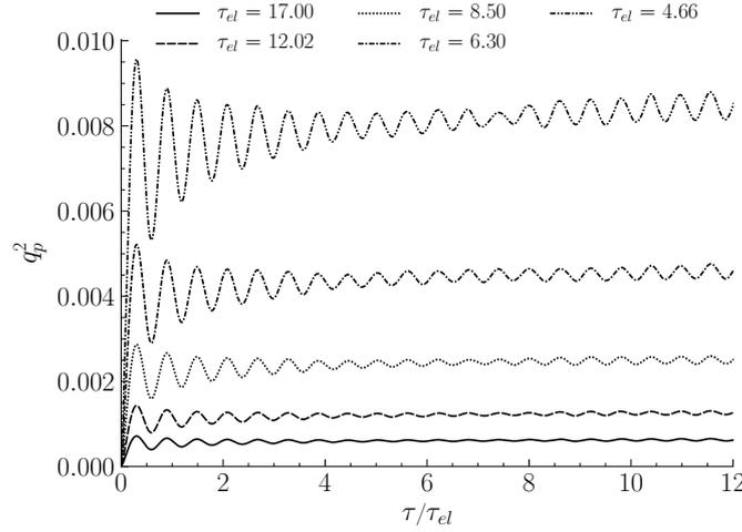
**Figure 4.23:** Time evolution of particle agitation for various levels of particle inertia.
