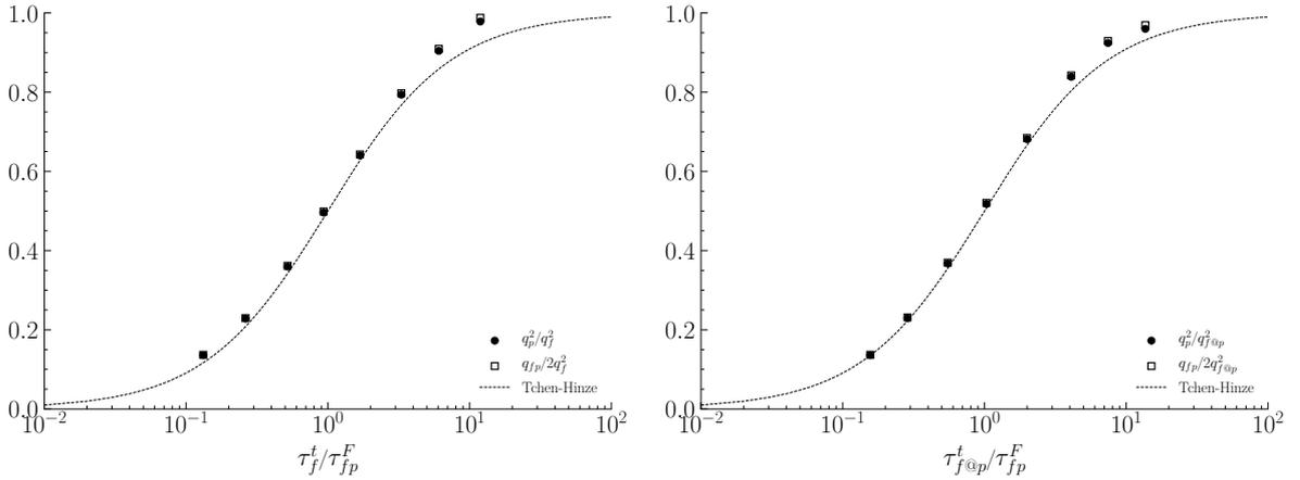
**Figure 3.1:** Particle agitation with regard to the inverse of the Stokes number. The dashed line corresponds to the Tchen-Hinze theory given by Eq. (3.10) (left) and its extension given by Eq. (3.9) (right). A good agreement of the DNS data with the two equations is observed.
