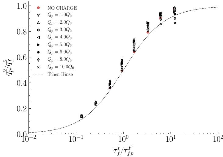
**Figure 5.5:** Effect of electrostatic interactions on particle agitation with regard to particle inertia for various levels of electric charge. The black dashed line corresponds to the Tchen-Hinze theory given by Eq. (3.10) and the red markers to the charge-free case.
