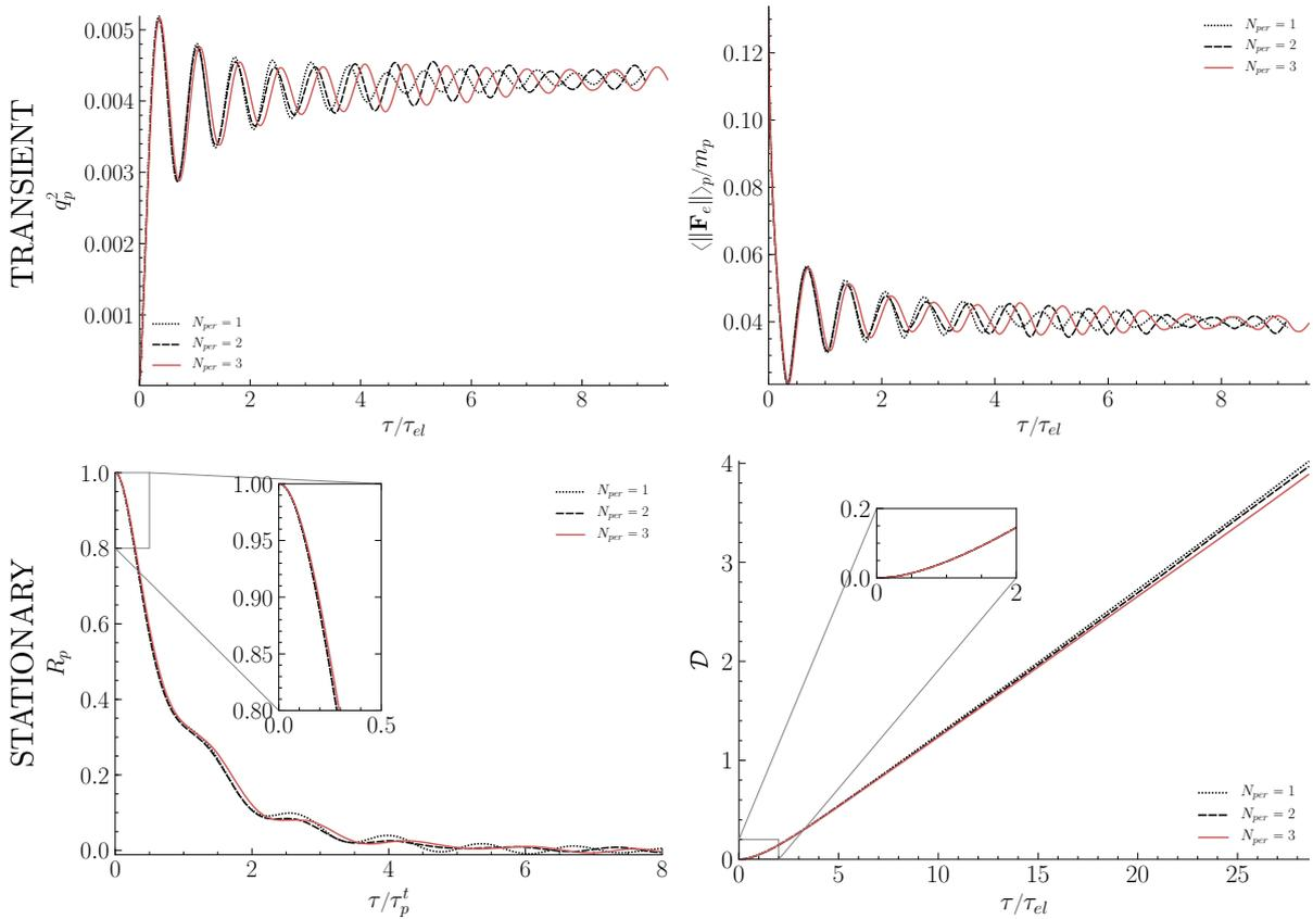
**Figure 4.8:** Evolution of particle agitation, Lagrangian particle velocity autocorrelation function, MSD and electrostatic acceleration for increasing number of periodic layers  $N_{\text{per}}$ . Convergence of statistics for the stationary regime is observed for  $N_{\text{per}} \geq 1$ .
