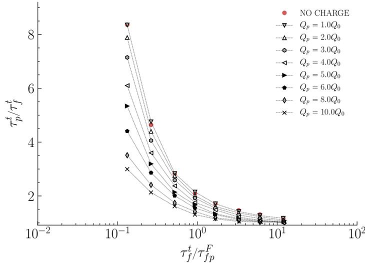
**Figure 5.24:** Effect of electrostatic interactions on  $\tau_p^t$  with regard to particle inertia for various levels of electric charge.
