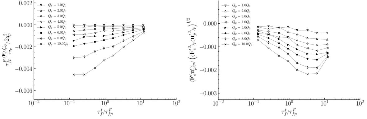
**Figure 5.7:** Effect of electrostatic interactions on term  $\langle \mathbf{F}'_e \mathbf{u}'_p \rangle_p / m_p$  with regard to particle inertia for various levels of electric charge.
