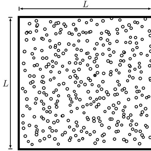
**Figure 4.2:** Computational domain of interest  $\Omega$  of length  $L$  contains  $N_p$  particles. A particle (black dot) interacts electrostatically with all  $N_p - 1$  other particles in the domain.
