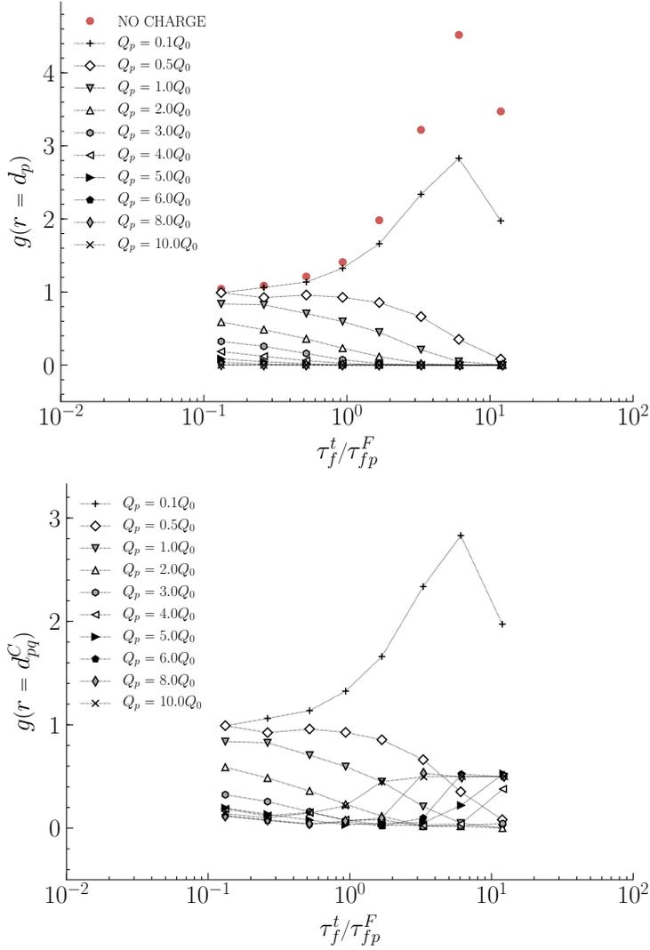
**Figure 5.43:** *RDF at separation distance  $r = d_p$  and  $r = d_p^C$  with regard to particle inertia for various levels of electric charge. The red markers correspond to the charge-free case.*
