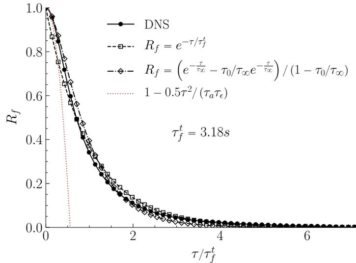
**Figure 2.6:** Autocorrelation functions of fluid velocity "seen" by fluid elements. Integration gives the Lagrangian fluid integral time-scale  $\tau_f^t$ . A good agreement with the exponential models is observed. The red dotted line denotes the oscillator function.
