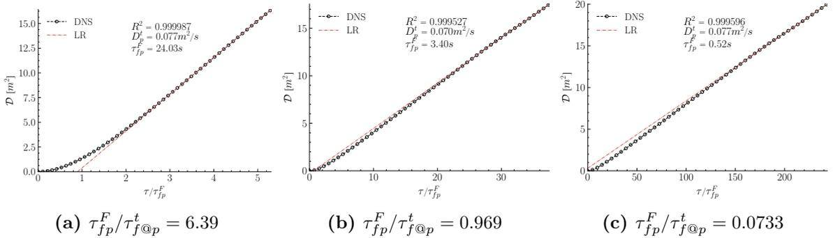
**Figure 3.11:** Mean squared particle displacement  $\mathcal{D}(\tau)$  with regard to  $\tau/\tau_{fp}^F$  for two Stokes numbers. A non-linear short-term and a linear long-term evolution is observed.
