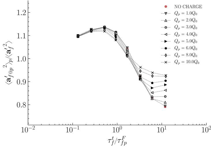
**Figure 5.14:** Effect of electrostatic interactions on fluid acceleration at the particles position  $\langle \mathbf{a}'_{f@p}{}^2 \rangle_p$  with regard to particle inertia for various levels of electric charge.
