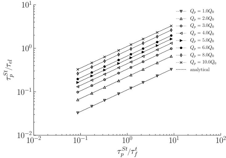
**Figure 5.1:** *Electrostatic Stokes with regard to the particle Stokes number for various levels of electric charge. Symbols correspond to the numerical simulation and the dashed lines to the analytical Eq. (5.2).*
