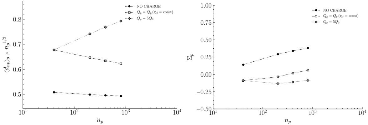
**Figure 5.54:** Effect of particle number density on particle distribution for different levels of particle charge. Nearest-neighbor particle distance (left), global particle accumulation (right).
