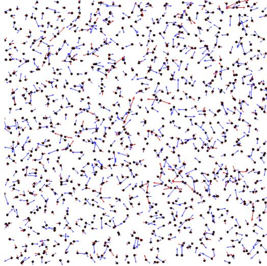
**Figure 4.22:** *Instantaneous snapshot of a dry like-charged particle cloud for  $\tau_{el} = 8.5s$  and  $\Delta x = L/10$ . Particle velocities are depicted with blue color, while electrostatic forces with red.*
