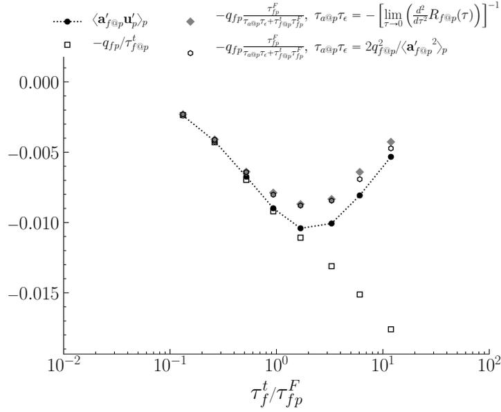
**Figure 3.9:** Comparison between DNS results ( $\bullet$ ) and the predictions of the Langevin model ( $\square$ ) as well as of the introduced stochastic model ( $\blacklozenge, \circ$ ) of  $\langle \mathbf{a}'_{f@p} \mathbf{u}'_p \rangle_p$  with regard to particle Stokes number.
