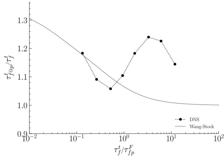
**Figure 2.10:** *Sensitivity of Lagrangian integral time scale of the fluid from the point of view of the particles with regard to particle response time. Semi-empirical model of Wang & Stock (1993) (see Eq. (2.50)) is also plotted for comparison.*
