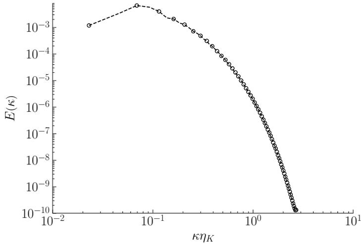
**Figure 2.2:** *Turbulent energy spectrum for  $Re_{L_f} \simeq 100$ .*
