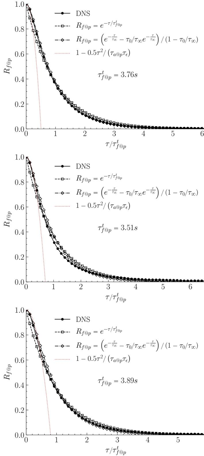
**Figure 3.8:** Autocorrelation functions of fluid velocity "seen" at the particle positions. Integration gives the Lagrangian fluid integral time-scale  $\tau_{f@p}^t$ . A good agreement with the exponential models is observed. The red dotted line represents the oscillator function.
