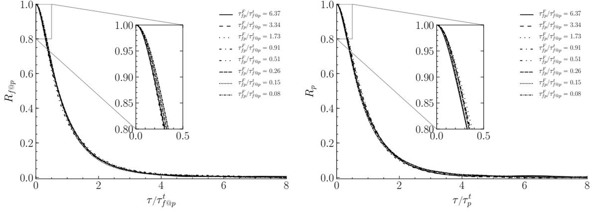
**Figure 5.20:** Autocorrelation function  $R_{f@p}$  of fluid velocity "seen" at the particle positions (left) and  $R_p$  of particle velocity (right) with regard to time normalized by corresponding integral time scale for various Stokes numbers in the case of  $Q_p = 5Q_0$ .
