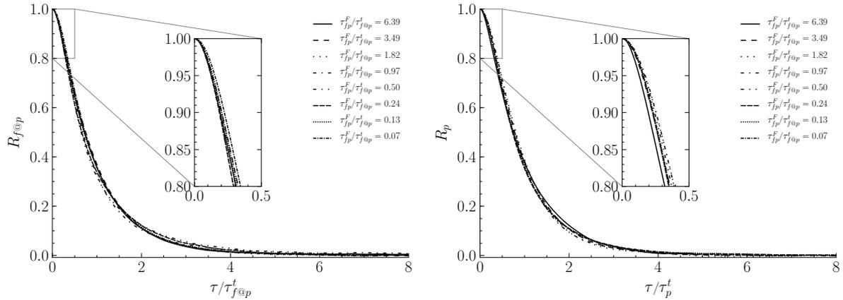
**Figure 2.9:** Autocorrelation function  $R_{f@p}$  of fluid velocity "seen" at the particle positions (left) and  $R_p$  of particle velocity (right) with regard to time normalized by corresponding integral time scale for various Stokes numbers in the charge-free case.
