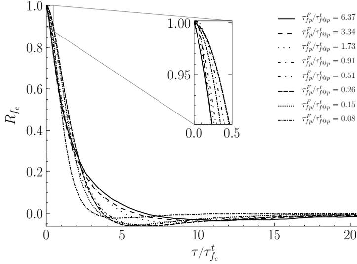
**Figure 5.34:** Autocorrelation functions of electrostatic forces,  $R_{f_e}$  with regard to time normalized by the corresponding integral time scale for various Stokes numbers in the case of  $Q_p = 5Q_0$ .
