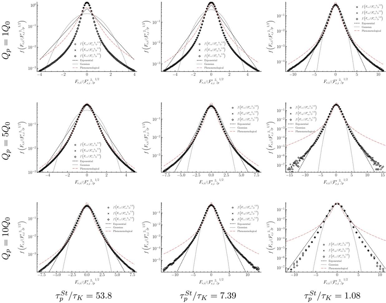
**Figure 5.30:** PDF of the three components of electrostatic forces for various levels of particle inertia and electric charge. The distributions are compared with the corresponding exponential and Gaussian distributions from Eq. (3.55) and the phenomenological ones from Eq. (5.13).
