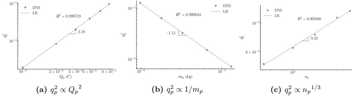
**Figure 4.18:** Particle agitation  $q_p^2$  for like-charged granular flow.
