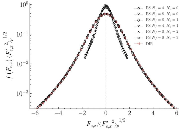
**Figure 4.15:** PDF of  $x$ -component of electrostatic forces for direct and pseudo-particle algorithm for various  $N_e$  with  $N_v \geq 0$ . Choice  $N_v = 0$  should be avoided as it leads to a substantial error in the calculation of particle electrostatic forces.
