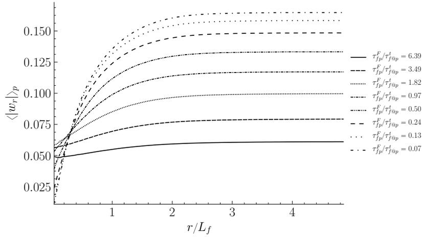
**Figure 3.25:** *RDF of average radial relative particle velocity in the charge-free case.*
