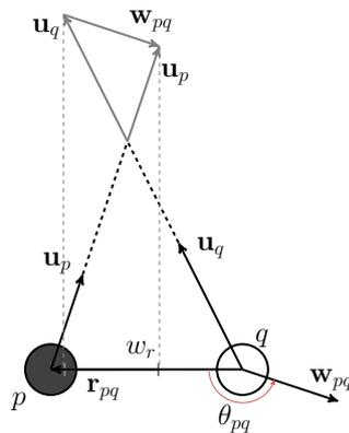
**Figure 3.24:** Notations for inter-particle relative motion.
