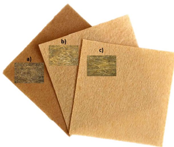
Fig. 3. Pictures and optical microscopy images (x10) of BF mats treated with a) 30%, b) 6% and c) 1% NaOH concentration.
