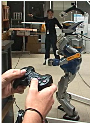
Fig. 3.9: Steering HRP-2 with a gamepad.
