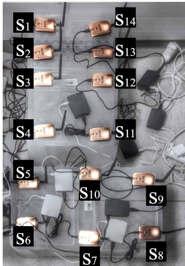
Figure 4.4. – Composition of the super-sniffer. The order in which we place our co-located sniffers to form a super-sniffer of maximum size 14.
