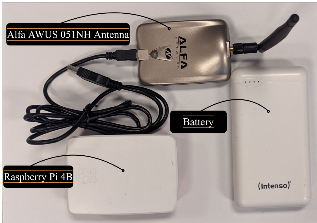
Figure 3.1. – A single sniffer. It is composed of a Raspberry Pi 4B node, an Alfa AWUS 051NH antenna, and an external power supply (20,000 mAH/74/0 Wh and 3.1 A output) to allow us to carry out the measurements for a longer period of time.
