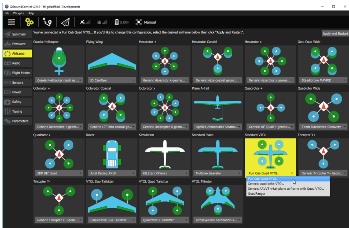
Figure 1.4: Examples of possible drone configurations considered by QGroundControl
