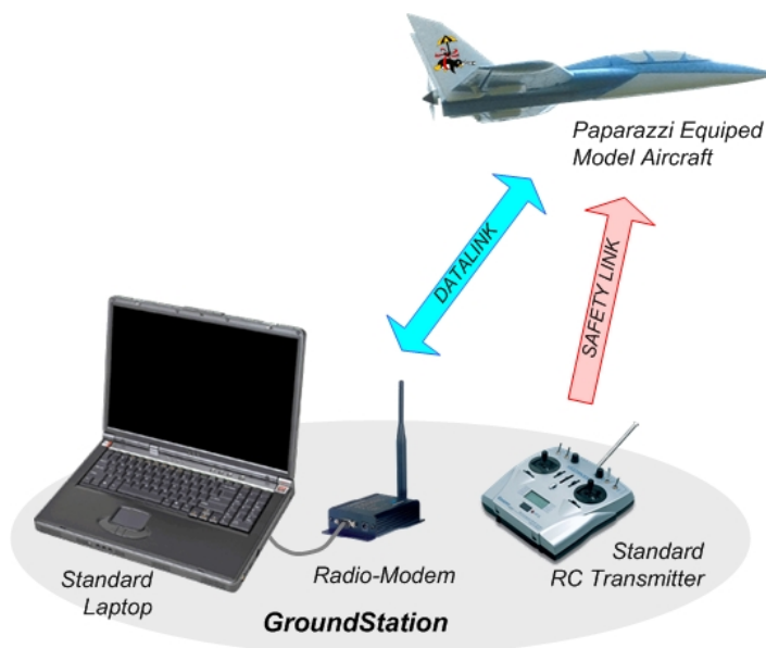
Figure 3.1: Paparazzi UAV simplified telemetry overview
