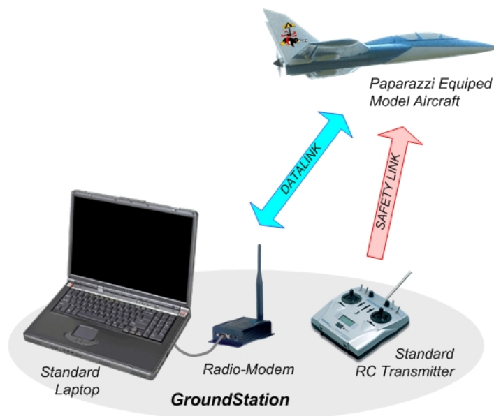
Figure 3.1: Paparazzi UAV simplified telemetry overview
