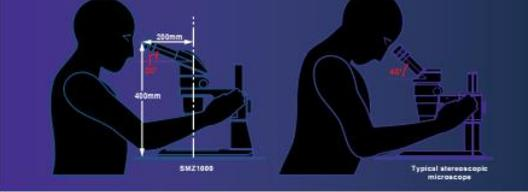
**Eyepiece tube inclination of 20°**
