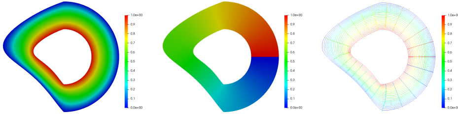
FIGURE 3.3 – Potentials \varphi_e (left) and \psi_m (center), associated isolines (right).
