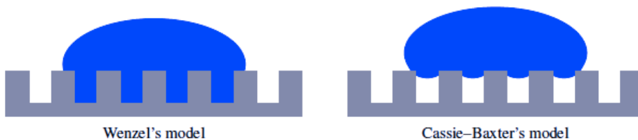
Fig. 1.14 A schematic description of the models proposed when a water droplet (blue) lies on a rough surface (in gray). Source: AD, designed with Tikz L A T E X package
