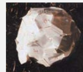
The model Smalley made with 60 vertices, 12 pentagonal and 20 hexagonal faces. Source: Kroto 1992, p. 117.
