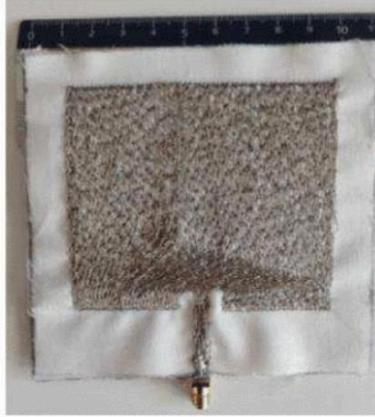
**Figure I-24.** Antenne textile [118]
