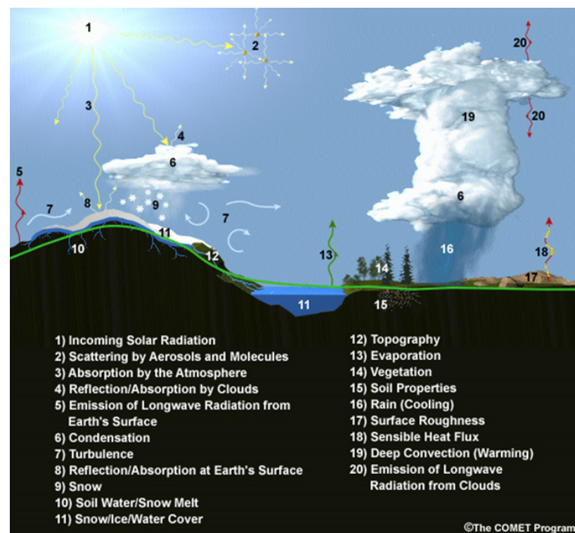
Figure 1.26: A list of 20 climate processes and properties that typically need to be parameterised within global climate models (from MetEd, The COMET Program, UCAR).
