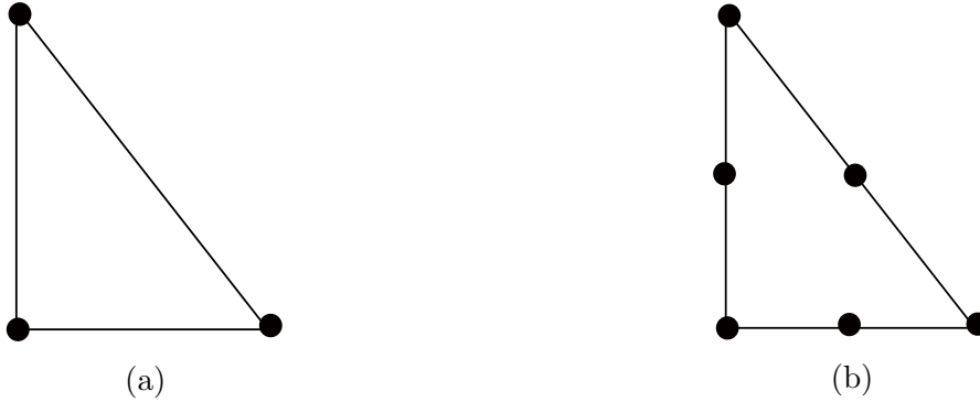
Figure 4.2 – Nodes of a canonical triangle for different degrees of precision. (a) Element \mathbb{P}_1 . (b) Element \mathbb{P}_2
