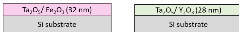
Figure 6.4: Tantalum-based thin films samples deposited on Si substrate. Left is \text{Ta}_2\text{O}_5 doped with \text{Fe}_2\text{O}_3 , and the right is \text{Ta}_2\text{O}_5 doped with \text{Y}_2\text{O}_3 .
