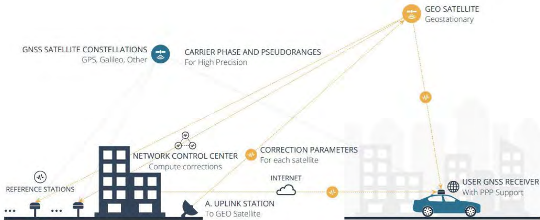
Figure 3-2 Precise Point Positioning [47]
