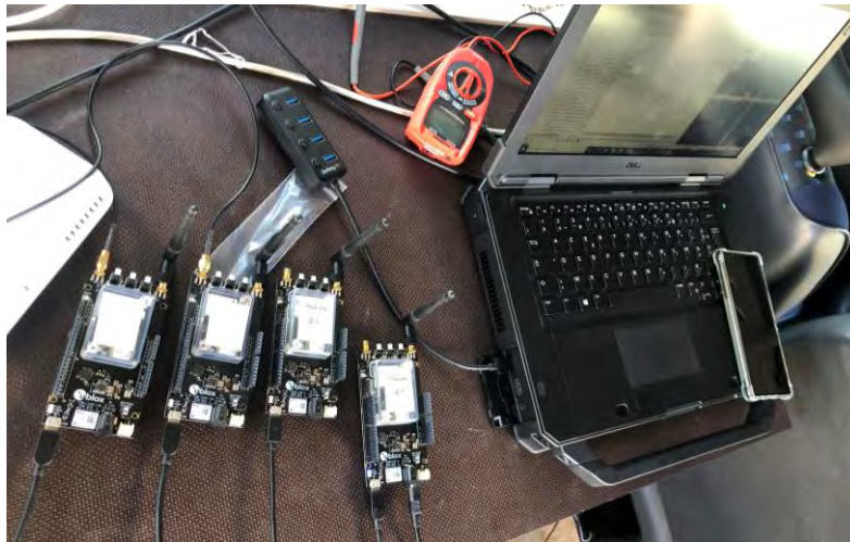
Figure 6-1 Illustration of the four U-blox GNSS receivers inside the vehicle
