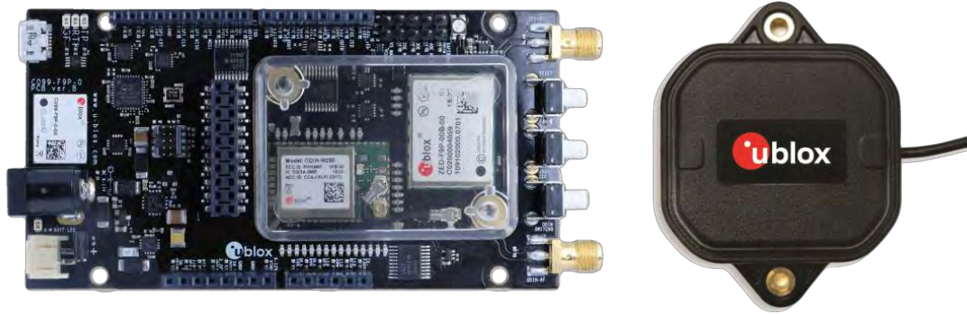
Figure 6-4 U-blox F9P GNSS Receivers (Left) and its magnetic ANN-MB series multi-band patch antenna (Right)
