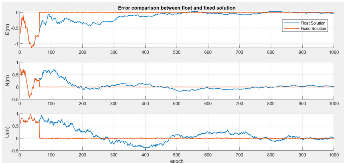
Figure 5-31 Illustration of float vs fixed solution (0 baseline)
