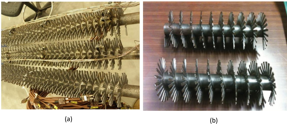
Figure 43. Photograph of the finned tube (a) prototype module (b) fraction of the tube's length
