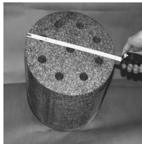
Figure 6. Single segment made of PCM/composite material used for the laboratory-scale storage unit. Holes are intended for steam pipes. [30]
