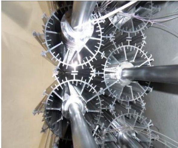
Figure 16. Photo of tubes with circular radial fins with metallic inserts constructed at CEA Grenoble
