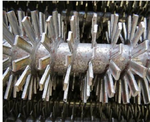
Figure 17. Photo of a tube with serrated radial fins constructed at CEA Grenoble
