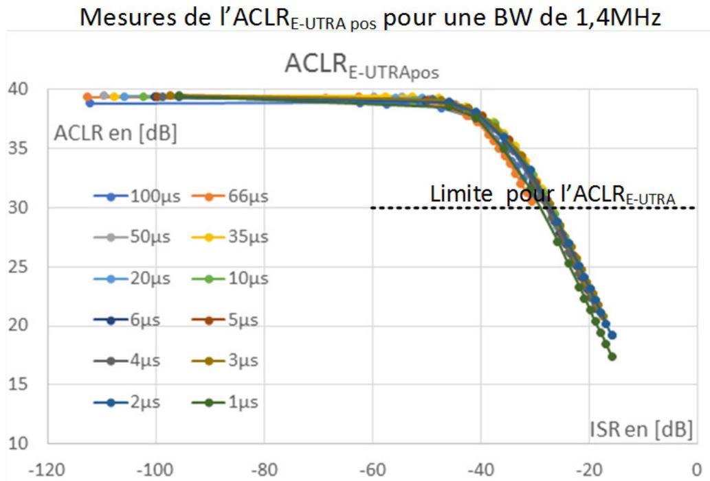
FIGURE 4.5 – ACLR<sub>E-UTRA pos</sub> BW = 1,4 MHz
