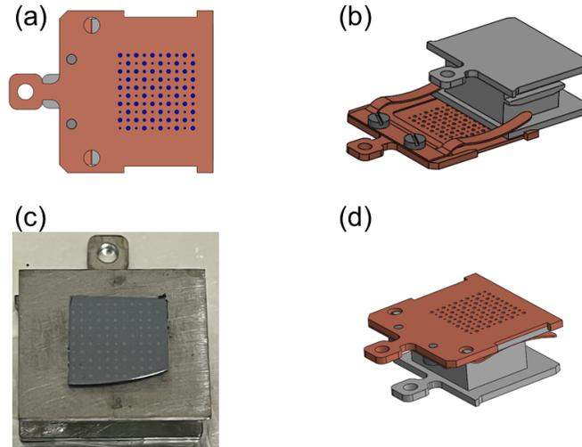
Figure 2.15: 3D design of (a) prepared shadow mask for BEEM measurements  $1 \times 1\text{cm}^2$  with 3 sizes of holes  $250\mu\text{m}$  ,  $350\mu\text{m}$  and  $500\mu\text{m}$ , (b) and (d) present placing the mask on the sample holder, and (c) a prepared sample with metallic Au dots.
