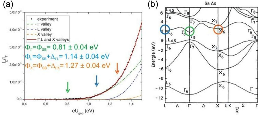
Figure 2.9: (a) Adjustment by the LP model, spectrum obtained on a junction  $Au(5nm)/GaAs(001)$  (average of 6400 curves for a surface of  $100 \times 100nm^2$  and (b) band structure of GaAs, figures taken from [53, 64].
