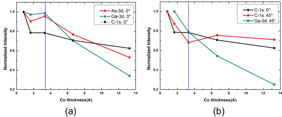
Figure 4.3: XPS study of different Co thicknesses on a grafted GaAs(001) substrate at RT(Mg- $\kappa$ ), all intensities have been normalized to their initial value at  $0.8 \text{ \AA}$  Co-thickness, (a) Ga-3d, As-3d and C-1s signal evolution with Co deposition at 0 degree, (b) C-1s evolution at 0 and 45 degree, Ga-3d evolution at 45° is presented as a reference of damping factor.
