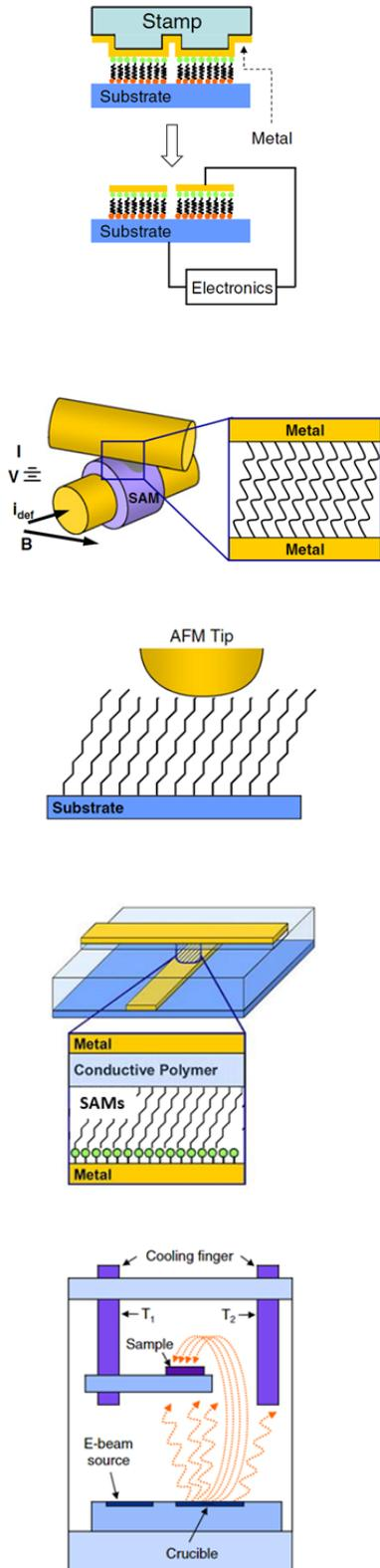
*Transfer printing:* a metal-coated stamp is brought into mechanical contact with a monolayer-coated substrate, with a reactive termination group. This high reactivity in regard to the metal adhesion to the stamp leads to a transferred pattern once removing the stamp.
