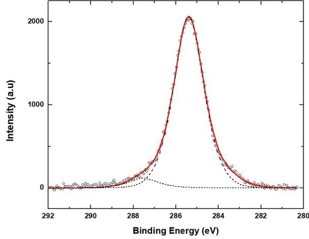
Figure 3.10: XPS spectrum, C16MT/Fe(001)/MgO/(001), C-1s peak is shown after grafting, measured with  $Al - k\alpha$  source. The major peak located at  $E_B = 285.3eV$  is assigned to C-C and C-H bonds, whereas a negligible signal is observed for C=O, 3eV shifted in binding energy.
