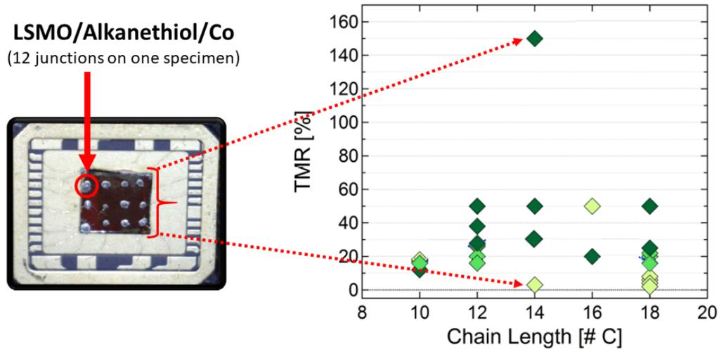
Figure 1.14: TMR measurements on *LSMO/Alkanethiol/Co* systems from C10, C12, C14, C16 and C18 (in the right), different TMR amplitudes have been detected from one specimen containing 12 junctions (in the left), figure is adapted from [26].
