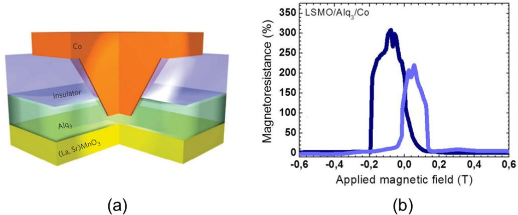
Figure 1.6: (a) Schematic structure of a nanometric-size MTJ of  $LSMO/Alq_3/Co$ , (b) MR curve measured of a  $LSMO/Alq_3(2nm)/Co$  junction at 2 K and -5 mV, Figure reprinted from [18].
