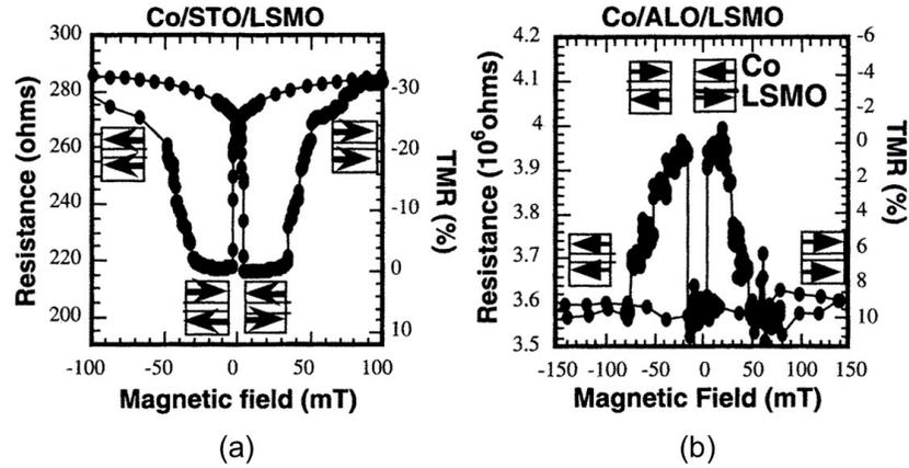
Figure 1.2: TMR curves obtained at bias voltage of  $-10\text{mV}$ , and at  $40\text{K}$  (a)  $\text{Co}/\text{SrTiO}_3(\text{STO})/\text{LSMO}$ , (b)  $\text{Co}/\text{Al}_2\text{O}_3(\text{ALO})/\text{LSMO}$  junction. Opposite signs TMR are observed with identical LSMO and Co ferromagnetic electrodes, Figures are reprinted from [11]
