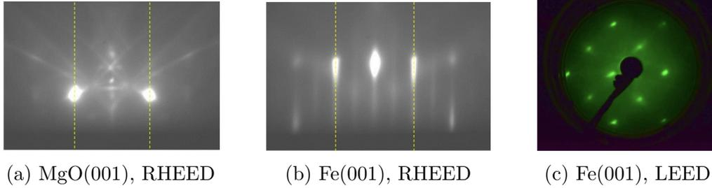
Figure 3.5: Fe(001) electrode, (a) MgO(001) substrate RHEED pattern, after annealing at 560°C for 1 hour (detection beam parallel to  $[110]_{MgO}$ ), (b) Fe(001)/MgO(001) RHEED pattern, 30nm Fe annealed at 560°C for 1 hour (detection beam parallel to  $[100]_{Fe}$ ). (c) Fe(001)/MgO(001) LEED pattern.
