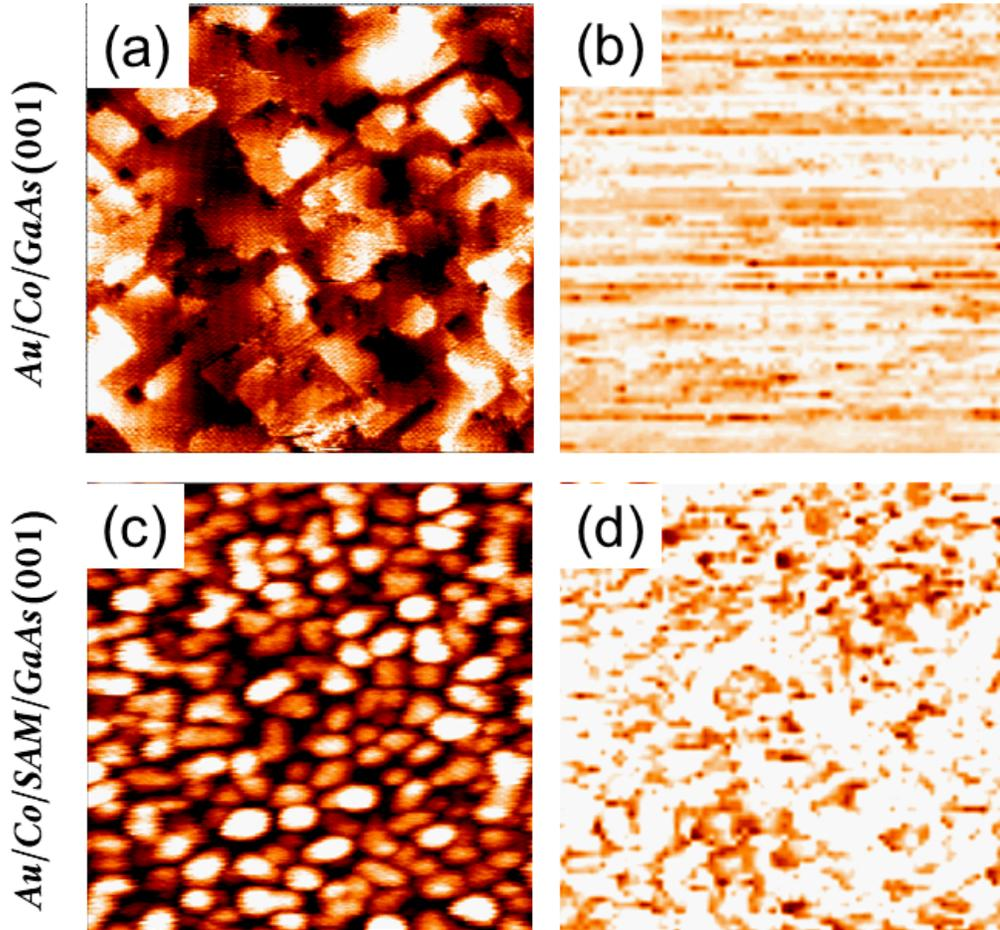
Figure 4.5: Room temperature specimens (a)STM image and (b) simultaneously recorded BEEM image of Au(4nm)/Co(3nm)/GaAs(001) at 1.8 V,  $I_T = 11nA$  (color scale: 10 to 50 pA),  $60 \times 60 nm^2$ . (c) and (d) STM and BEEM images of Au(4nm)/Co(3nm)/C16MT/GaAs(001) at 1.75 V,  $I_T = 15.3nA$  (color scale: 40 to 80 pA),  $75 \times 75 nm^2$ .
