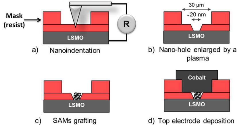
Figure 1.13: Schematic of a *LSMO/SAM/Co* device fabrication. (a) Nanoindentation lithography technique: LSMO spin-coated with a resist which is indented by an AFM tip to form a nanohole, (b)  $O_2$  plasma is used to enlarge the nanohole to a final diameter of 10-50 nm, (c) SAM grafting process: immersing the sample in a SAM solution, (d) Co top-electrode deposition by sputtering. figure is reprinted from [26]
