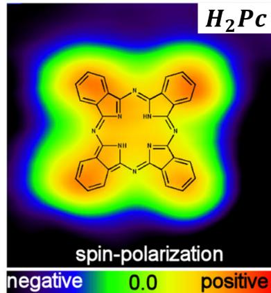
Figure 1.8: Spin polarized scanning tunneling microscopy experiment employed to image the spin polarization of a  $H_2Pc$  molecule deposited on an iron surface at 6K. The opposite surface spin polarization of iron (negative) and spin polarization above the molecule (positive) highlights the spin polarization inversion on the  $H_2Pc$  orbitals, figure is reprinted from[20].
