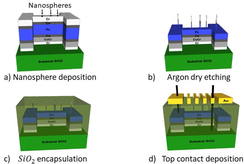
Figure 1.15: Schematic of a  $SiO_2//Cr/CoCr/Co/Pc/Co/Cr$  device fabrication by Nanosphere lithography technique. (a) nanosphere deposition on the surface, (b) Ar etching: tailoring the nanopillars protected by the shadow-masking nanospheres, (c) Passivation layer deposition: it serves to electrically decouple the parallel pillars with the same common bottom electrode (this layer is removed from the nanospheres using  $N_2$  gun), (d) Top-electrode deposition, figures are adapted from [47].
