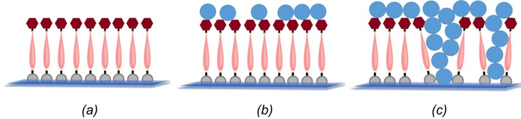
Figure 1.11: Schematic top-electrode deposition onto a grafted substrate, a) grafted substrate by SAM, b) formation of metal top-electrode, c) metal diffusion due to high kinetic energy of metal atoms through SAM.
