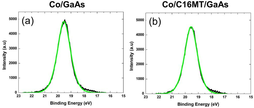
Figure 4.4: XPS study of Ga-3d evolution after Co deposition for thicknesses of 12Å, using BLAG method, (a) Co/GaAs(001) and (b) Co/C16MT/GaAs(001).
