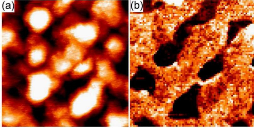
Figure 2.10:  $50 \times 50 \text{ nm}^2$  STM images of gold overlayer surfaces on SAM, Au/C16MT/GaAs(001)((a) 5 nm thick gold deposited at room temperature, with peak-to-peak roughness of 1.1nm. (b) Simultaneously recorded BEEM images at  $U_{gap} = 1.80V$  and  $I_T = 5nA$  (color scale: 0 to 0.16 nA), figures are taken from [53].
