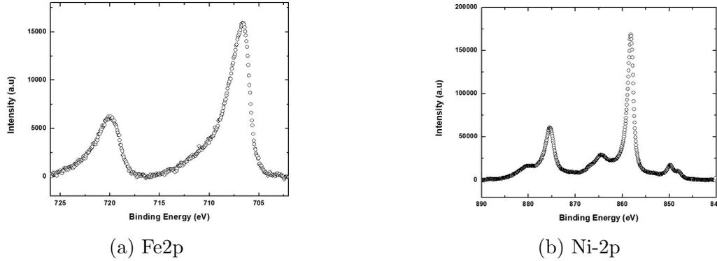
Figure 3.3: XPS spectra of Permalloy electrode measured with Mg- $k\alpha$  source(MgO(001)/NiFe), (a) Fe-2p $_{1/2}$  and Fe-2p $_{3/2}$  located at 719.9eV and 706.8eV, respectively. This location for Fe-2p core levels are reported for a metallic Iron layer, (b) Ni-2p.
