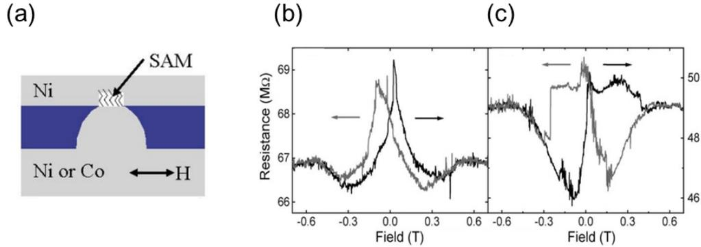
Figure 1.5: (a) Schematic structure of molecular MTJ using SAMs, (b) and (c) different resistance behaviour measured of two *Ni/octanethiol/Ni* junctions as a function of in-plane magnetic field at 4.2 K with a bias of 10 mV, Figures are reprinted from [17].
