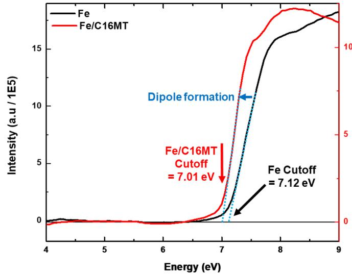
Figure 3.16: Low Intensity X-ray Photoemission Spectroscopy (LIXPS) using  $Al - k\alpha$  source, LIXPS-cutoff of Fe (black line) and Fe/C16MT (red line), leading to a dipole formation of  $\Delta_{LIXPS} = \Phi_{Fe} - \Phi_{SAM} = 0.10 \text{ eV}$ , by LIXPS.
