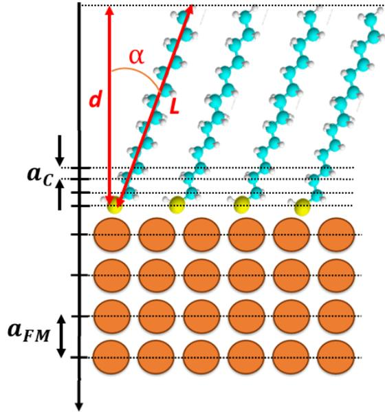
Figure 3.8: Schematic sketch of SAM grafted on a ferromagnet layer,  $a_{FM}$  and  $a_C$  are associated to the atomic distance between two layers of FM and C, respectively,  $d$  and  $L$  to the thickness and length of the molecules with a tilting angle of  $\alpha$ .
