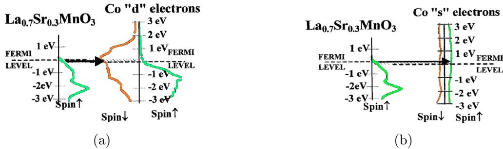
Figure 1.3: DOS of LSMO and Co, for d- and s-character electrons, the arrow represent the most probable tunneling transition (a) *STO/Co* interface selects d-bands of Co resulting in a negative TMR. (b) *Al<sub>2</sub>O<sub>3</sub>/Co* interface would select s-bands of Co resulting in a positive TMR. Figure reprinted from [11].
