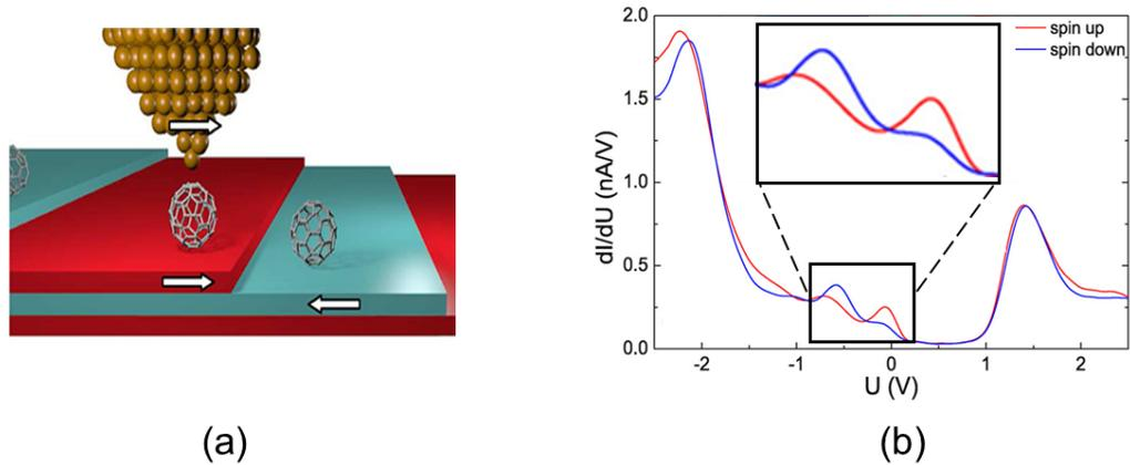
Figure 1.9: Spin-polarized scanning tunneling spectroscopy measurements on a  $C_{60}$  molecule deposited on a chromium surface. (a) Schematic view of the STM junction. (b) The difference in the conductance curves for the spin up (red) and down (blue) shows a spin dependent energy shifting of the molecular levels up to 0.5 eV, figure is reprinted from [19].
