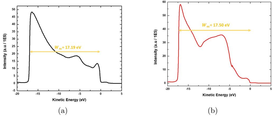
Figure 3.14: UPS spectrum using  $He I$  line,  $h\nu = 21.21 eV$ , (a) Fe layer,  $\Phi_{Fe} = 4.02 eV$ , (b) grafted Fe by C16MT  $\Phi_{SAM} = 3.71 eV$ , leading to a dipole formation of  $\Delta_{UPS} = \Phi_{Fe} - \Phi_{SAM} = 0.31 eV$ , by UPS.
