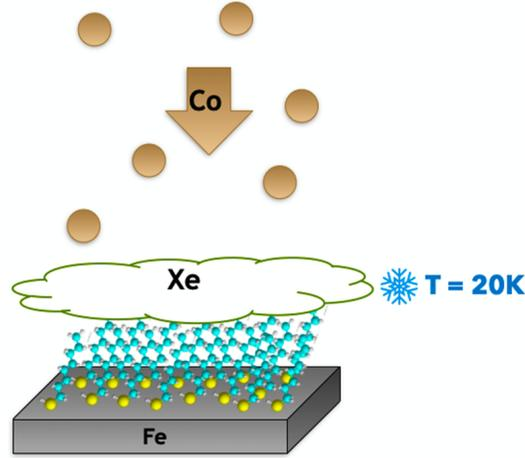
Figure 4.1: Schematic of top-electrode deposition employing BLAG technique.
