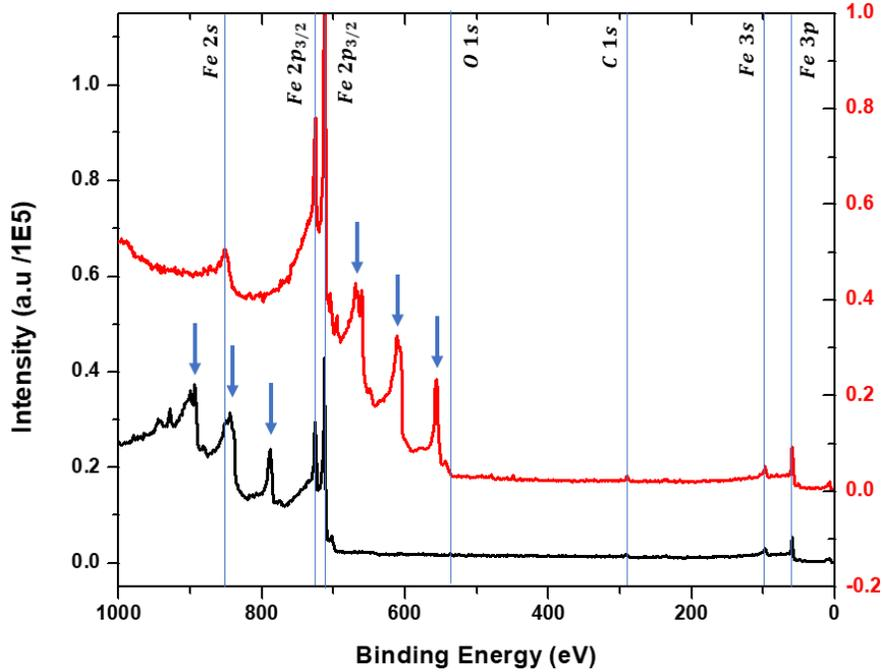
Figure 2.3: XPS spectra of Fe/MgO(001), with Al-K $\alpha$  (black line) and Mg-K $\alpha$  (red line) sources, Fe Auger peaks are marked with blue arrow observed with two sources, Fe, O and C core levels have been indicated by blue lines.
