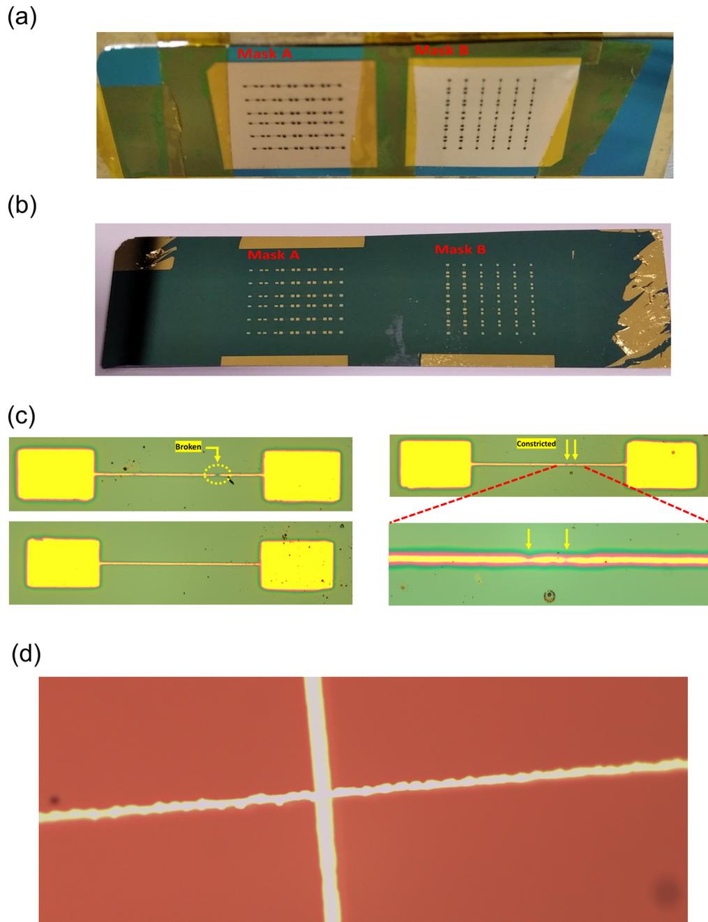
Figure 5.4: (a)  $\text{CuBe}_2$  shadow mask, Mask A with the thickness of  $t_{\text{mask}A} = 50$ , and mask B  $t_{\text{mask}B} = 20\mu\text{m}$  (b) 110nm Au deposition through the Mask A and mask B, (c) Optical images of a broken and a complete strip with the width of  $w = 10\mu\text{m}$  on mask A, (d) Optical images of a strip containing a zoom-in constriction,  $w = 5\mu\text{m}$ .
