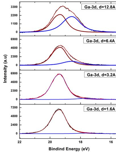
Figure 4.2: XPS study of Ga-3d evolution after Co deposition for thicknesses of  $d = 1.6, 3.2, 6.4$  and  $12.8 \text{ \AA}$  (red and blue fitting curves are attributed to Ga-3d core level and GaCo component, respectively).
