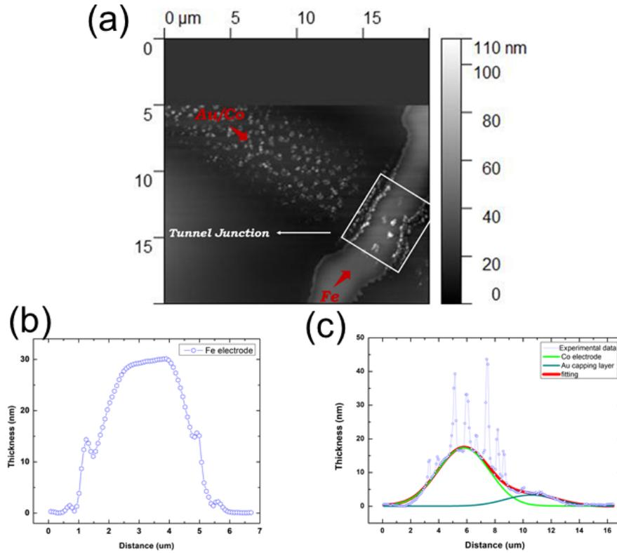
Figure 5.6: (a)  $20 \times 20 \mu\text{m}^2$  AFM image of the Fe and Au/Co electrodes, the *Au/Co/C16MT/Fe* tunnel junction is located at this intersection, shown in white square, (b) and (c) present a profile line of Fe and Au/Co electrode, respectively.
