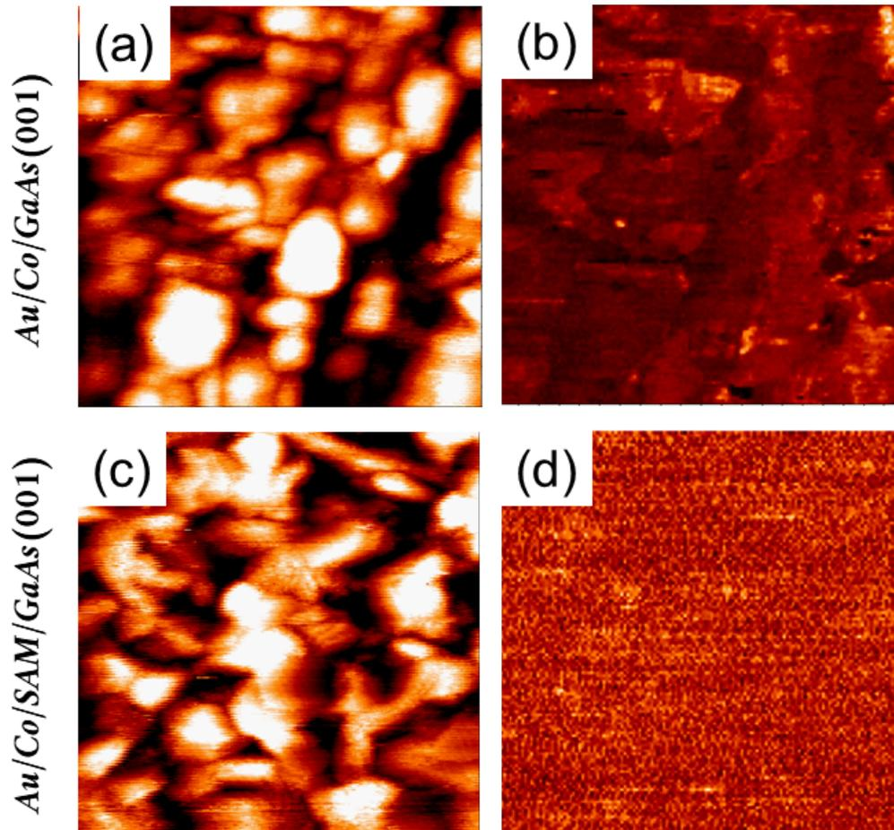
Figure 4.7: BLAG specimens (a)STM image and (b) simultaneously recorded BEEM image of Au(4nm)/Co(3nm)/GaAs(001) at 1.82 V,  $I_T = 15nA$  (color scale: 85 to 110 pA),  $100 \times 100 nm^2$ . (c) and (d) STM and BEEM images of Au(4nm)/Co(3nm)/C16MT/GaAs(001) at 1.81 V,  $I_T = 10nA$  (color scale: 16 to 20 pA),  $100 \times 100 nm^2$ .
