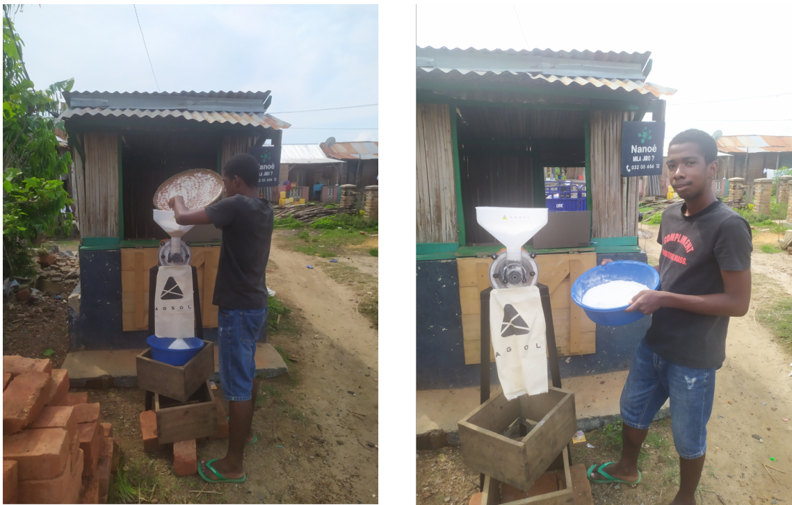
Figure IV.15: Rice milling with a communal load on the microgrid.
