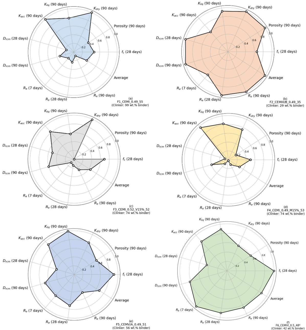
Figure II-40 Ratio of relative differences between MC and DC compared to the maximum obtained on the six formulations for F1 (a), F2 (b), F3 (c), F4 (d), F5 (e) and F6 (f).
