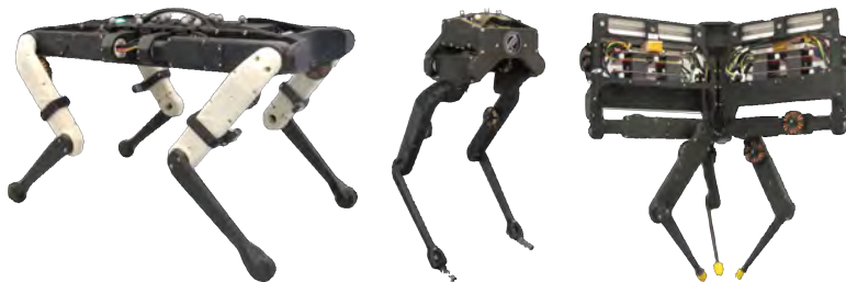
Figure 24: Different robots sharing the same modular actuator from the ODRI project [98]
