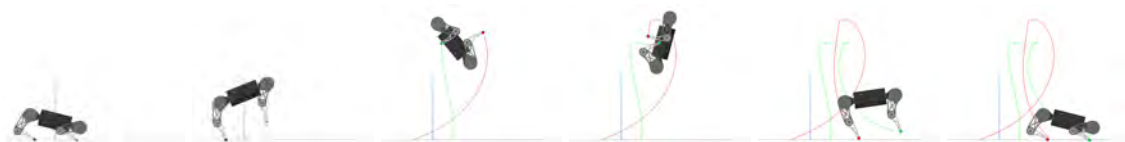
(a) Backflip movement: a full base rotation is required, the state trajectory is cyclic except for the x-translation. The robot must additionally also have zero joint velocity at the extremes of the trajectory.
