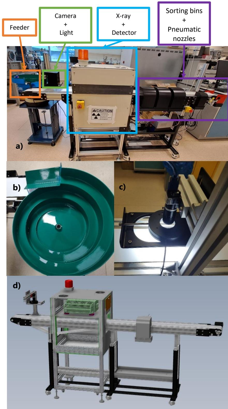
Figure 1: a) Photograph of the whole prototype, close view of the bowl feeder, c) close view of the camera and light and d) 3D CAD view of the prototype
