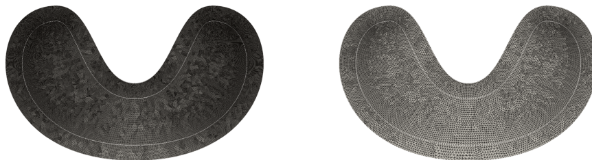
Figure 3.7: Representation of the mesh of \Omega with 56193 degrees of freedom (left) and with 14169 degrees of freedom
