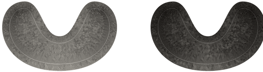
Figure 4.8: Representation of the mesh of \Omega with 14169 dofs (left) and with 56193 dofs (right)
