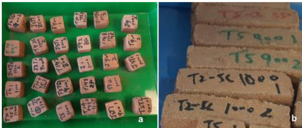
Figure 3. 16. Usumacinta bricks cubic (a) and prismatic specimens (b)
