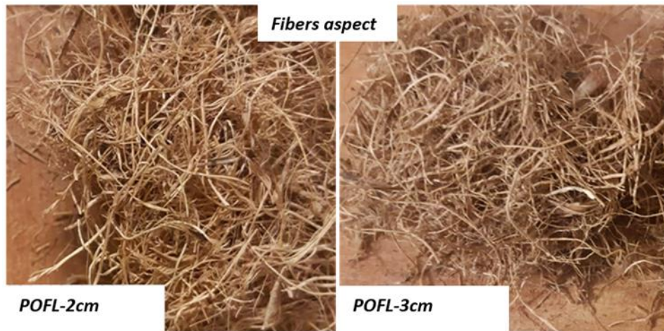
Figure 4. 13. POLF fiber of lengths G-2cm and G-3cm
