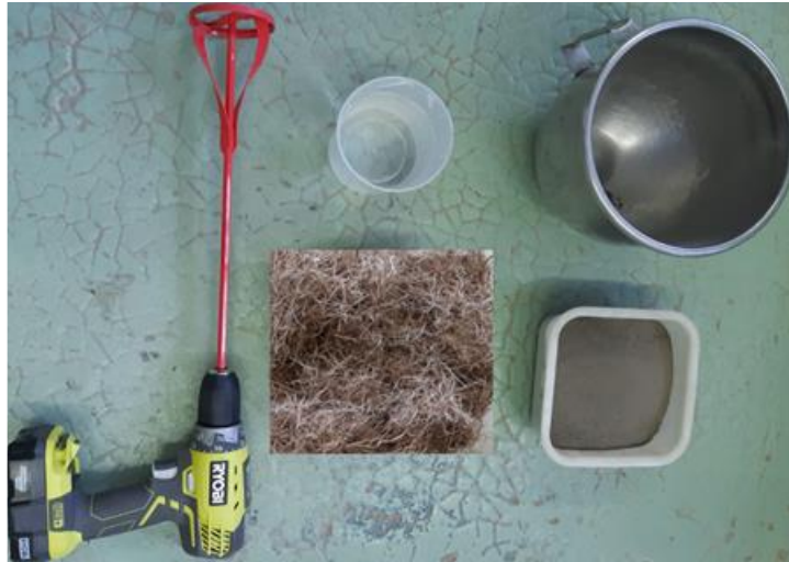
Figure 4. 16. Usumacinta River sediments and POFL fibers
