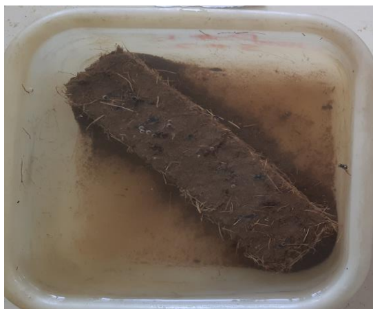
Figure 4. 29. Adobe brick immersion in water
