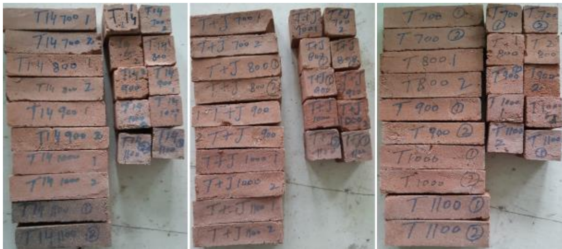
Figure 3. 19. Color variation with firing temperature in Usumacinta bricks
