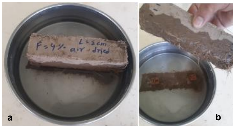
Figure 4. 28. Capillarity water absorption test
