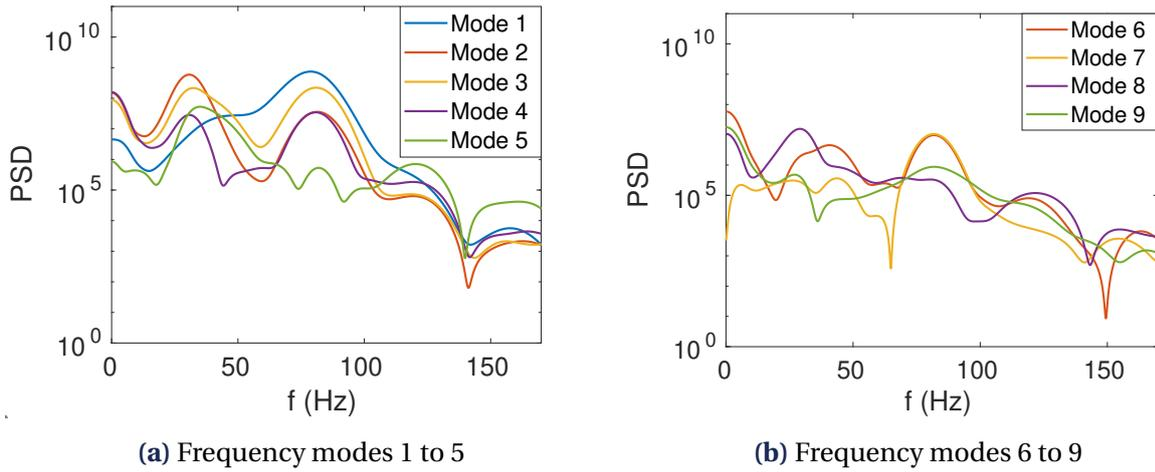
**Figure 3.18** • Power Spectral Density of the nine estimated PGD modes for the beam solicited with load 2 - bi-frequency load with  $f_a = 40\text{ Hz}$ ,  $f_b = 80\text{ Hz}$  at  $U_d^{\text{max}} = 30\text{ mm}$
