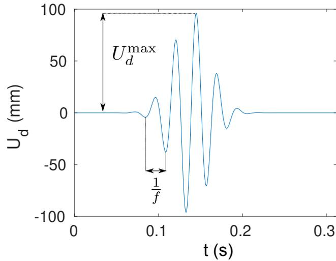
Figure 3.6 • Temporal load 1 - mono-frequency case
