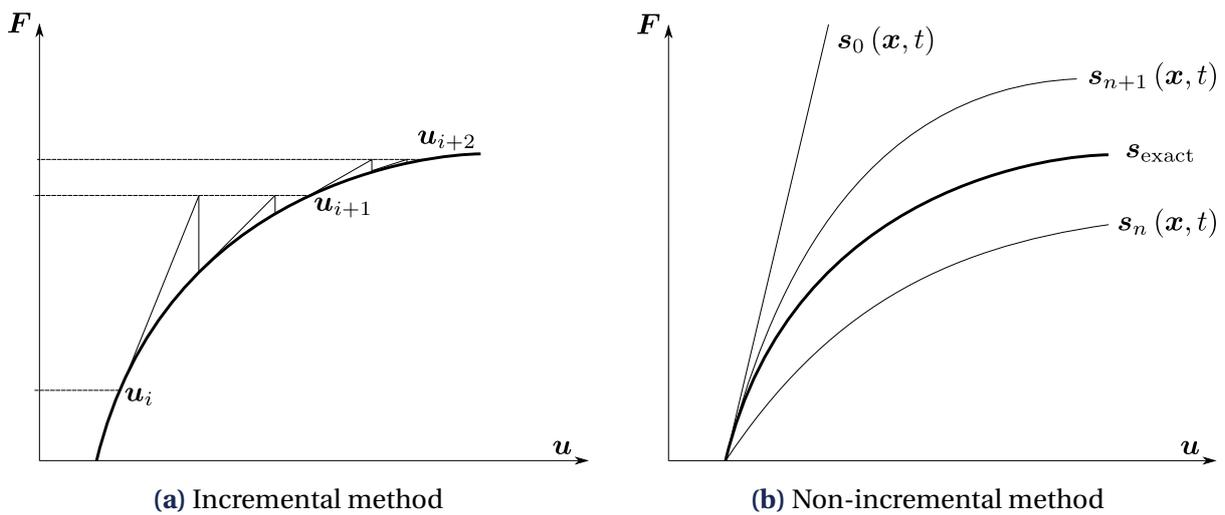
Figure 1.8 • Comparison between incremental and non-incremental schemes
