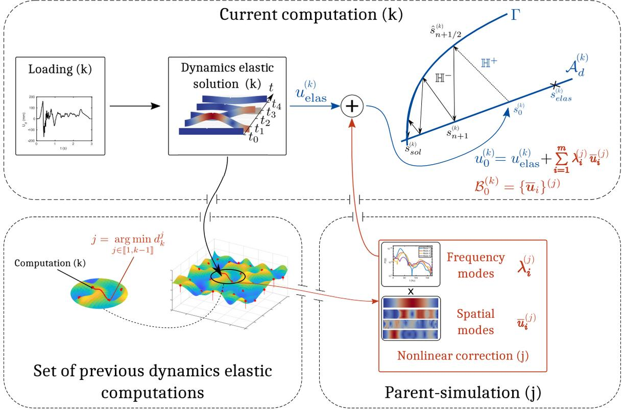
**Figure 4.3** • Computation ( $k$ ) enhanced from a chosen parent-simulation
