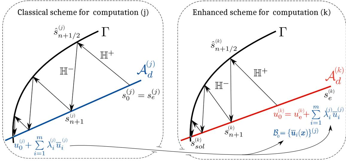
**Figure 4.2** • Standard and enhanced non-linear LATIN-PGD schemes
