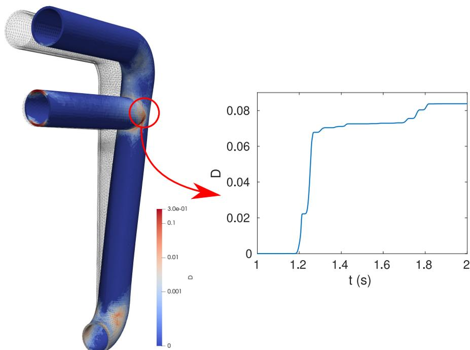
**Figure 3.27** • Damage field in the three-dimensional pipe structure solicited with a complex load at time  $t = 2$  s and damage evolution at the T-junction between the tube and the middle branch over time
