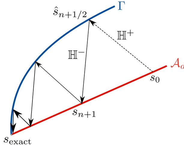
**Figure 3.1** • Working principle of the LATIN method, modified from [Ladevèze, 1999]
