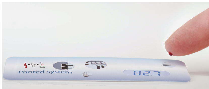
Figure 3: Example of a quantitative POC giving glucose concentration from a blood drop via an amperometric sensor [1].
