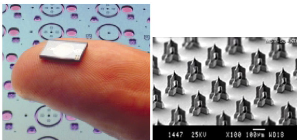
Figure 4: Implantable device based on MEMS (left) Micropump developed by Debiotech SA for insuline, injecting 150nL per cycle; The system is patched over the skin of the insulin dependent patient (right) SEM picture of integrated MEMS needles for injection [2].
