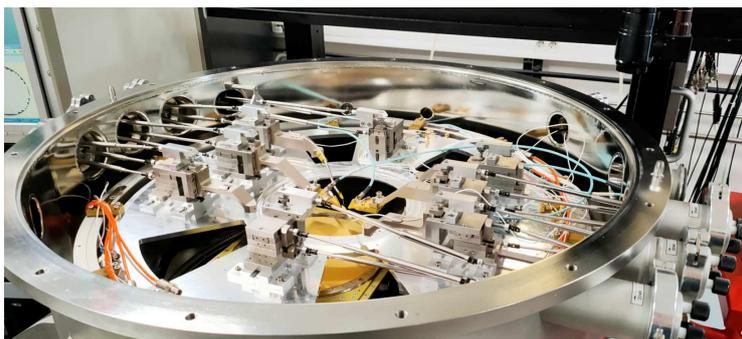
Figure 3.22: View of the inside of the vacuum chamber of the PAV2000 prober.
