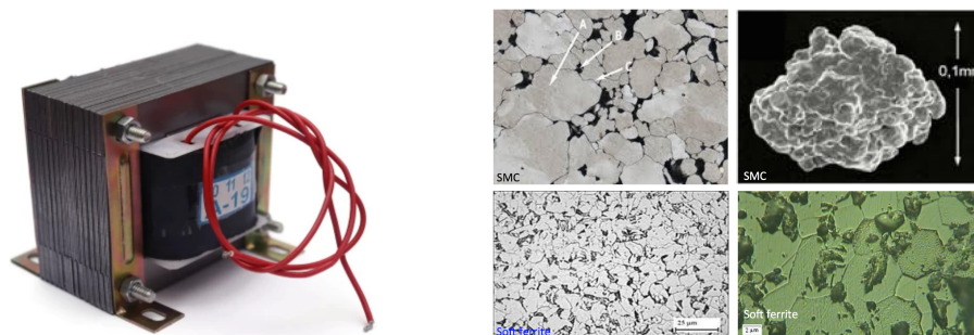
Figure 0.1: Electric transformer with laminated magnetic core (left) and magnetic composites (right)
