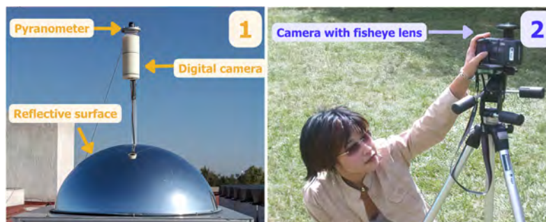
Figure 1.8: Reflective dome technique (1) [31] and fisheye camera imaging (2) [32]
