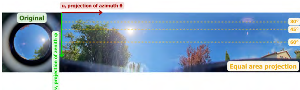
Figure 1.23: Illustration of the transformation from fisheye photo to an equal-area projection of the demi-sphere.
