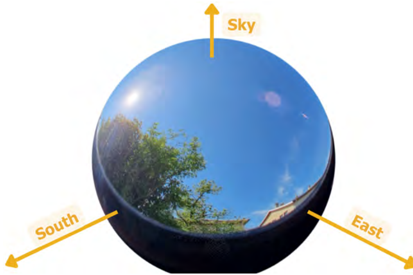
Figure 1.22: Illustration of how the diffuse shading factor should be calculated properly. We need to consider the area of shading over the total area of the sky on the surface of a sphere, not on a flat image. This image was taken by determining the equivalent azimuth and zenith of each pixel and it is then mapped onto a unit sphere.
