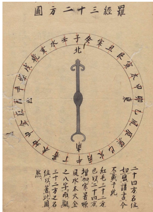
Figure 3.7. Model of a compass ( rakyō 羅經) with the “thirty-two directions of the Dutch” ( kōmō sanjūni hō 紅毛三十二方) as depicted in Nishikawa Joken’s Ryōgi shūsetsu (National Archives of Japan)
