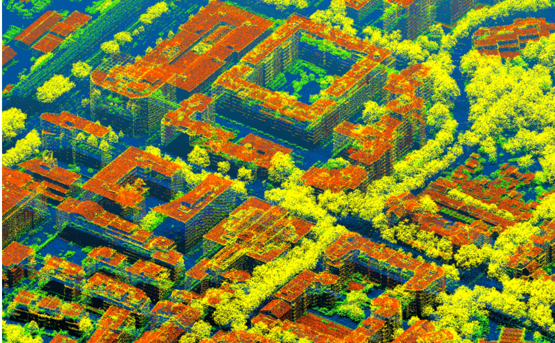
Fig. 1.2 Aerial LiDAR 3D point cloud of the 6 th arrondissement of Lyon, acquired in 2015 with a density of 12 points/m 2 . The different colors correspond to the point classifications (i.e. vegetation in yellow, roofs in orange, façades in blue). Source: Métropole de Lyon website 1
