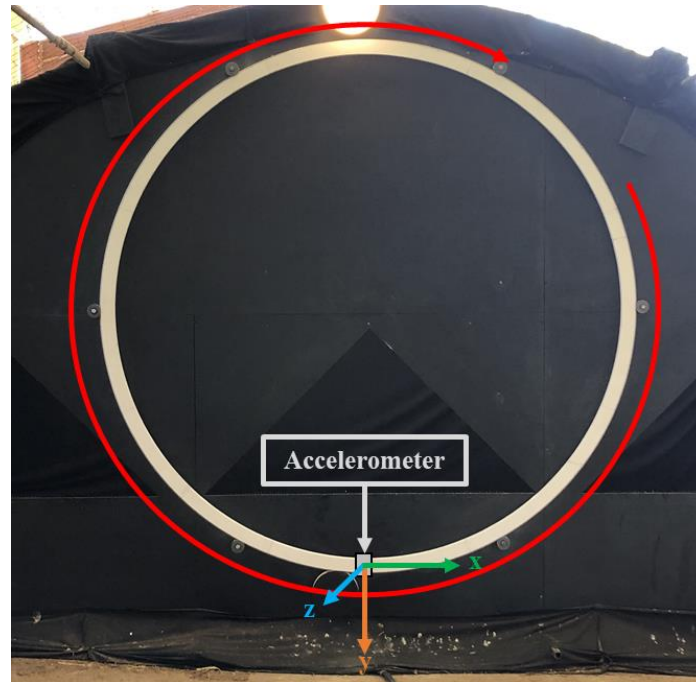
Figure S1. Using of accelerometer to measure wind turbine's speeds.
