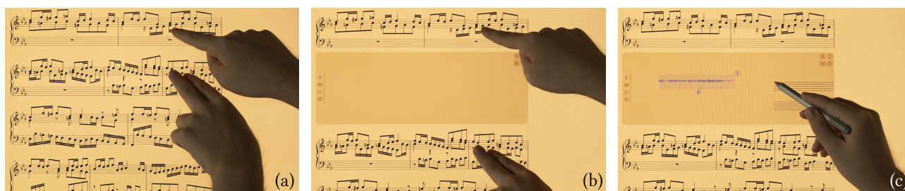
Figure 4.6: Carving a pensieve by (a-b) stretching space between two staves using a simple multitouch gesture, and then (c) populating that space with multiple objects using drag-&-drop. An audio sample has been dropped already, and the user is about to place an empty staff to write music on.
