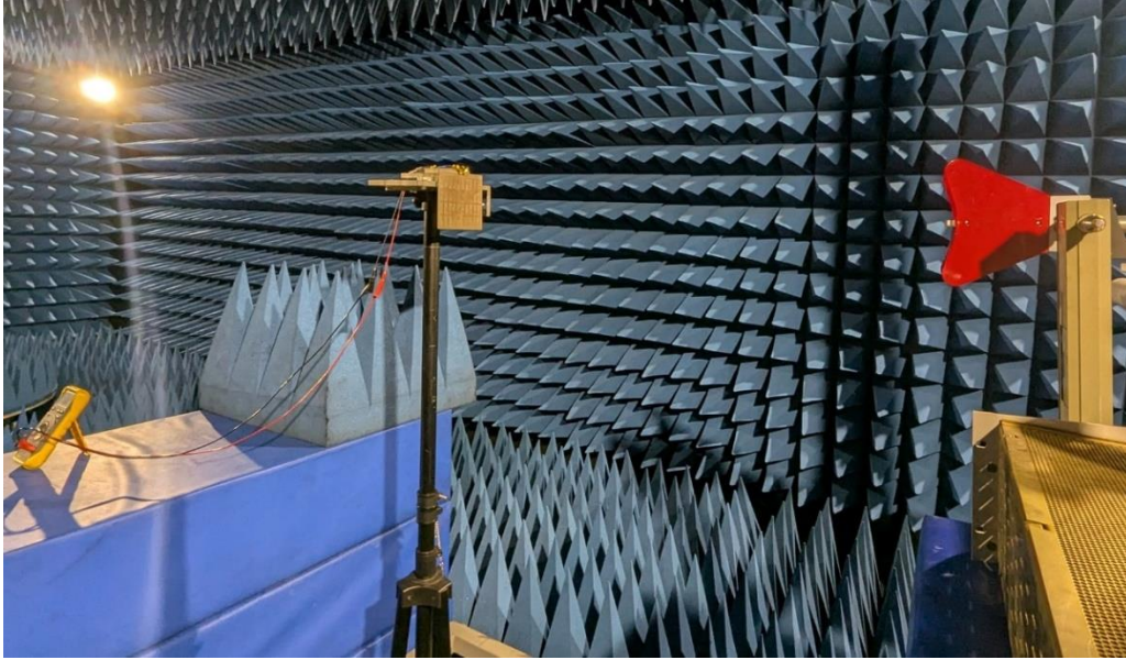
Figure 3.20 Measurement setup of the whole device in the anechoic chamber.
