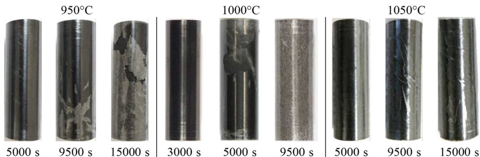
Figure 1.4 – Post-quenching appearance of Zircaloy-4 cladding samples two-sided oxidized in steam at 950 °C, 1000 °C and 1050 °C (Le Saux et al., 2020).
